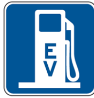
D9-11b Electric Vehicle Charging
