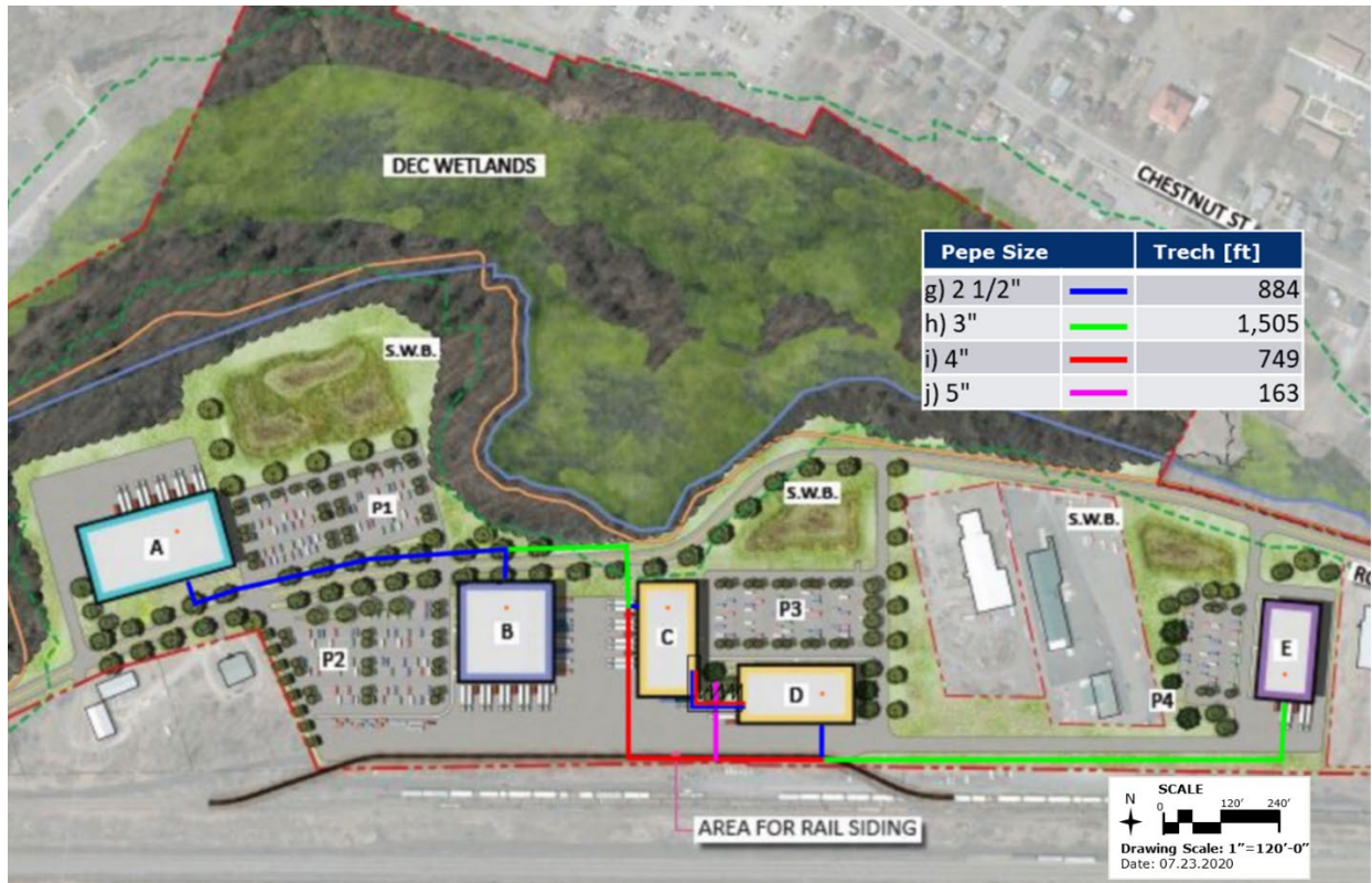
Figure 18. Proposed Low-Temperature Hot Water Network for Scenario 1
