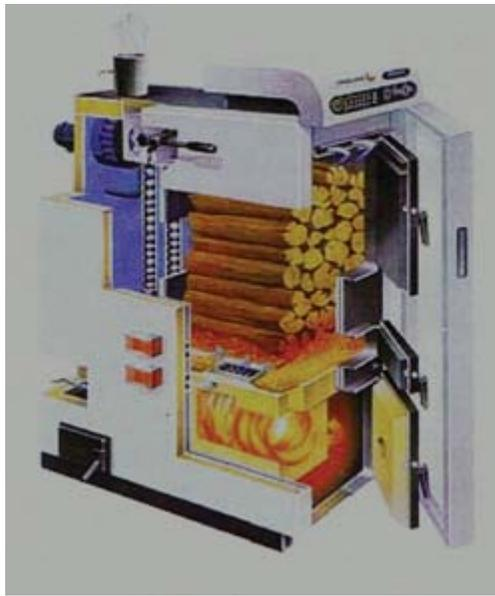
**Figure 3. Two-stage, split-wood, down-draft gasification boiler (Froeling, 2005).**
