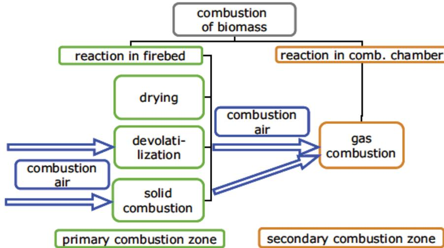
Figure 4. Process schematic of two stage combustion (NYSERDA, 2010).
