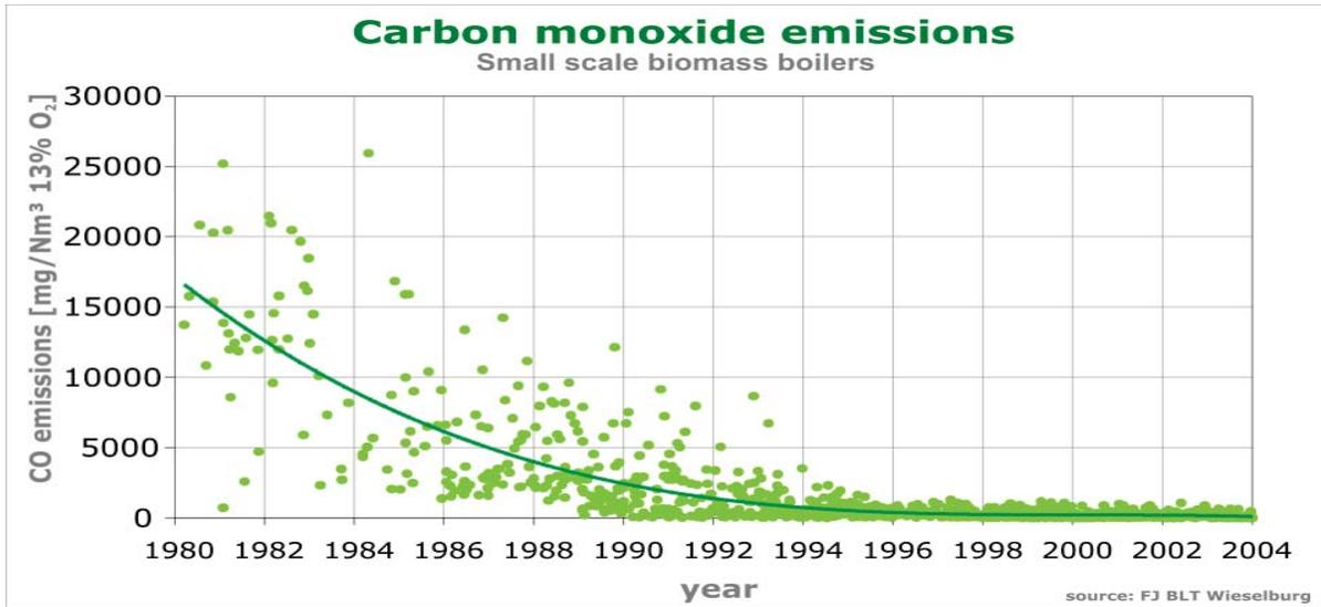
Figure 7. Carbon monoxide emissions drop from 15,000 to < 50 mg/m<sup>3</sup> over 25 years (Voglaur, 2005).
