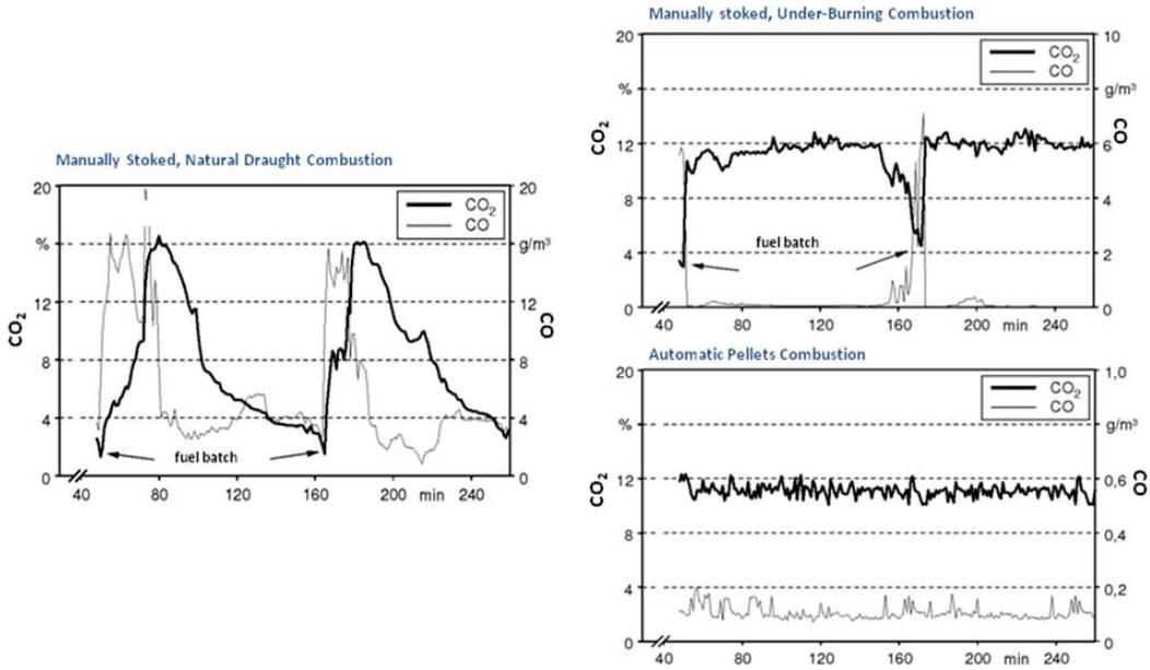
Figure 5. Comparisons of real-time CO/CO<sub>2</sub> emissions for through combustion, two-stage split wood, and 2-stage pellet boiler combustion performance (Hartmann, 2003).
