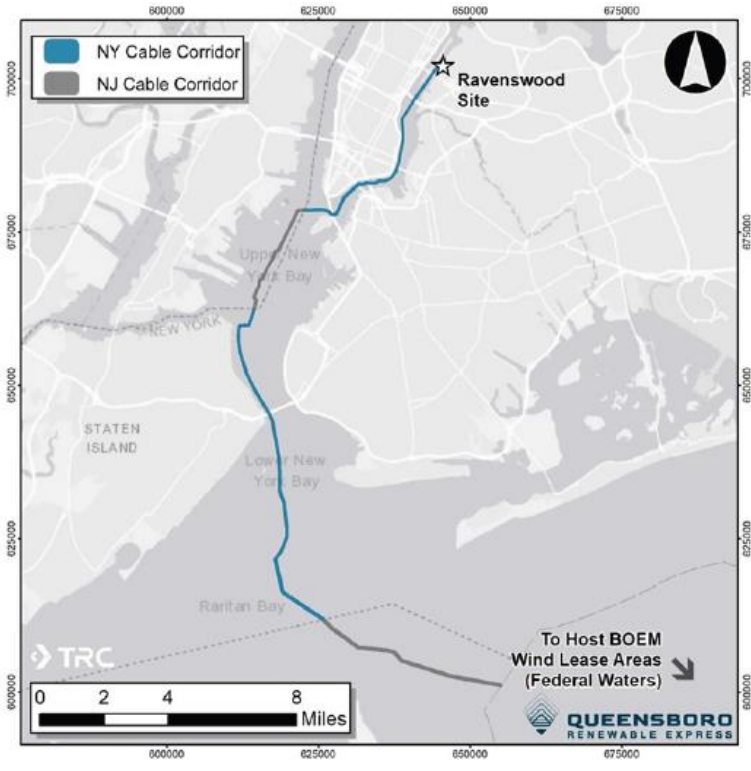
Figure 7-1. Export Cable Corridor through State Waters as Proposed in the Queensboro Renewable Express NYS Article VII Application
