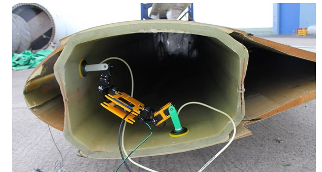
BladeBUG robot operating in confined spaces.
