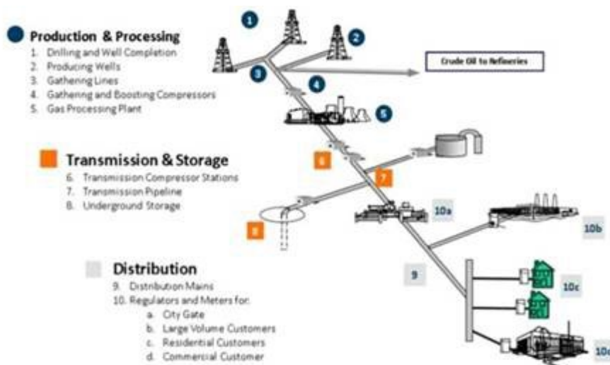
Figure 1: Basic Diagram of Natural Gas Distribution System
