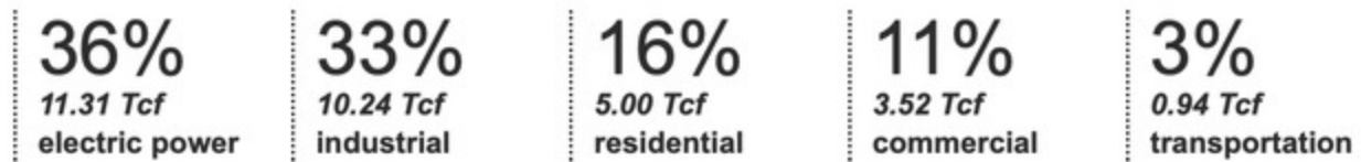
Natural gas use by U.S. consuming sectors by amount and share of total U.S. natural gas consumption in 2019
