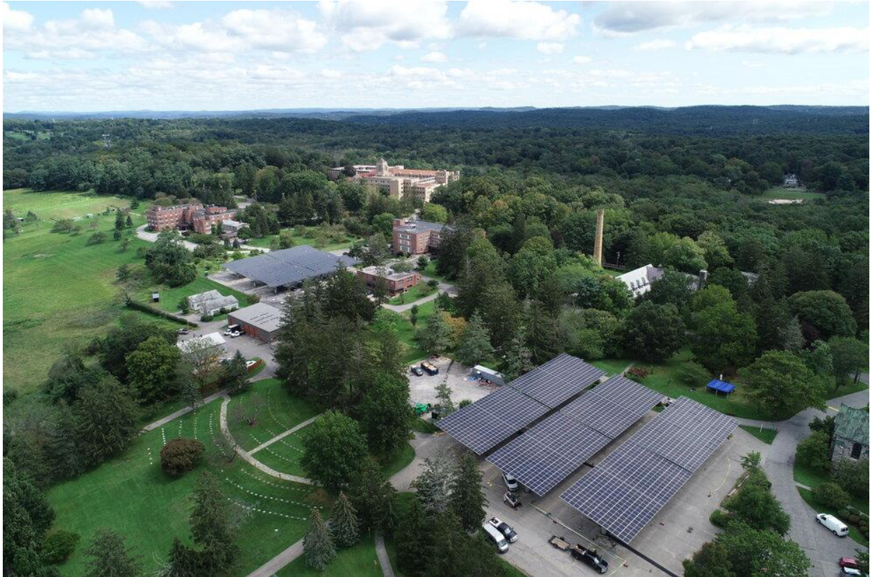
Figure 3. Ecogy's 873.6 kW DC system consists of 12 parking lot canopies hosted by the Maryknoll Fathers and Brothers of Ossining.
