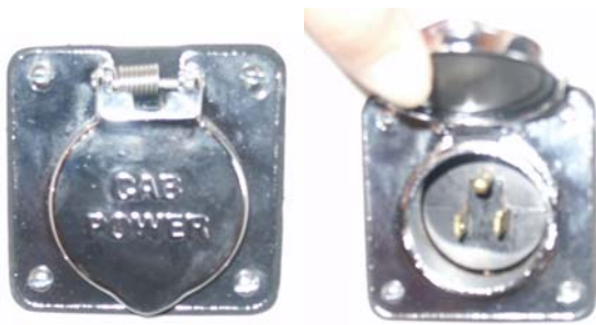
Figure 10. Block heater receptacle mounted on driver's side fender
