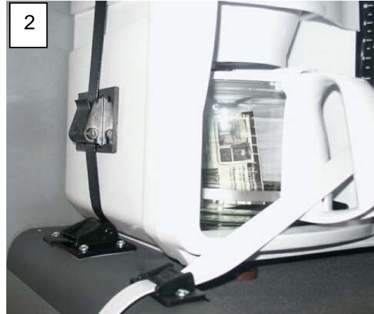
Figure 41: Space saver coffee pot mounted with RV-type securing straps
