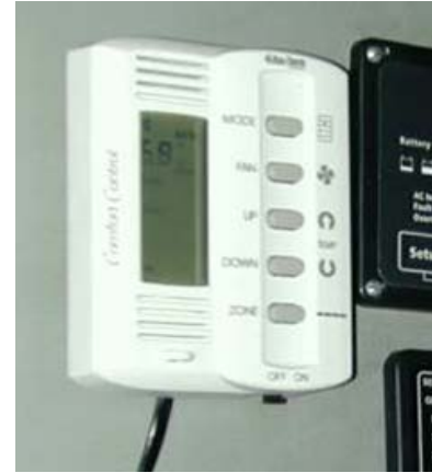
Figure 8: HVAC unit remote control panel
