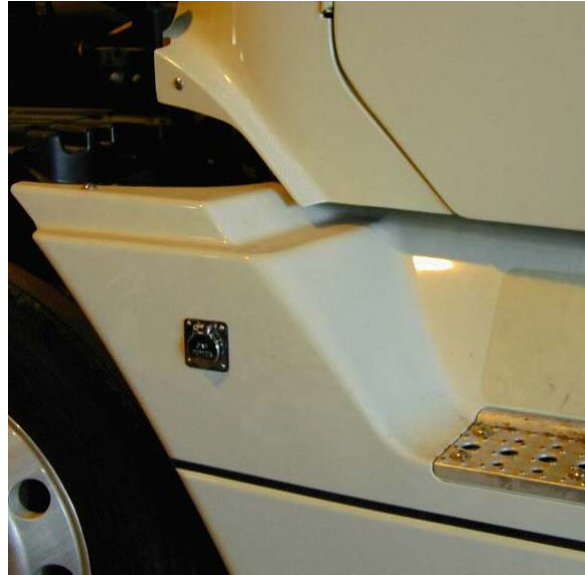
Figure 28: Phillips & Temro block heater outlet installed on driver's side step/fender
