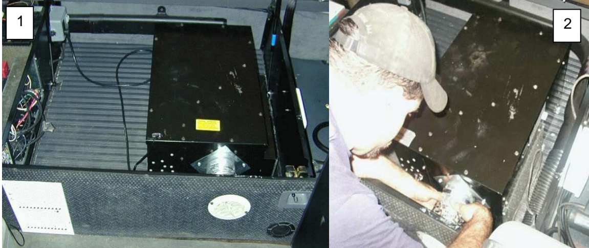
Figure 2: Installed Cab Comfort HVAC unit (left); Installation of optional flexible 4" air outlet ducting
