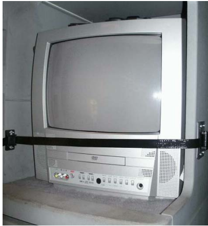
Figure 40: TV secured with mounting strap
