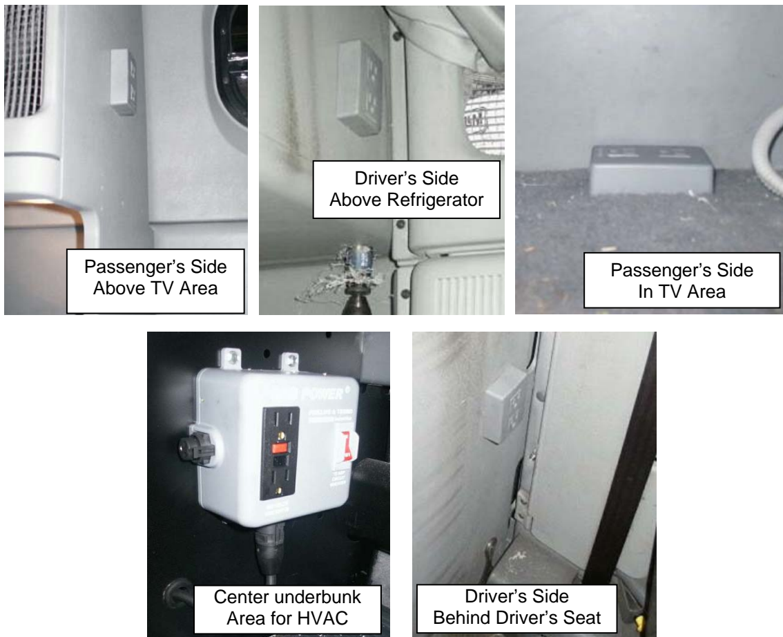
Figure 25: Interior surface mounted electrical outlet locations
