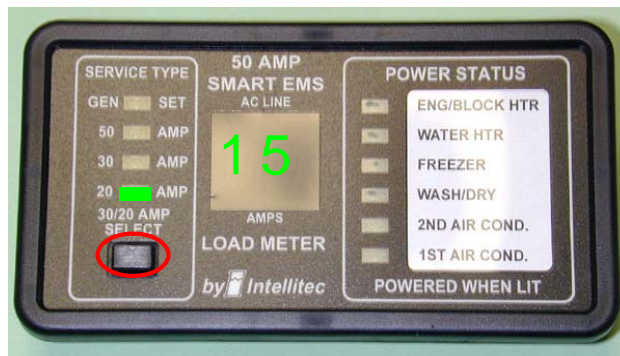
Figure 7. Smart EMS Display. 30/20 AMP SELECT button circled in red
