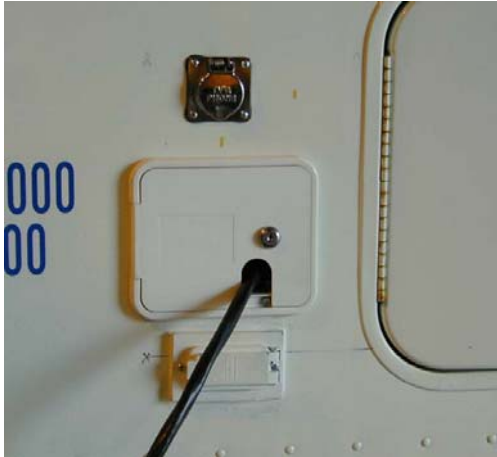
Figure 30: Exterior Shorepower outlets (from top to bottom: TV/phone, main power, and Internet)
