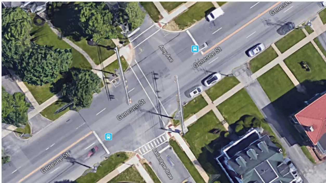
Figure 9. Details of Offset Intersection on Genesee Street at Ballantyne Brae and Amy Avenue
