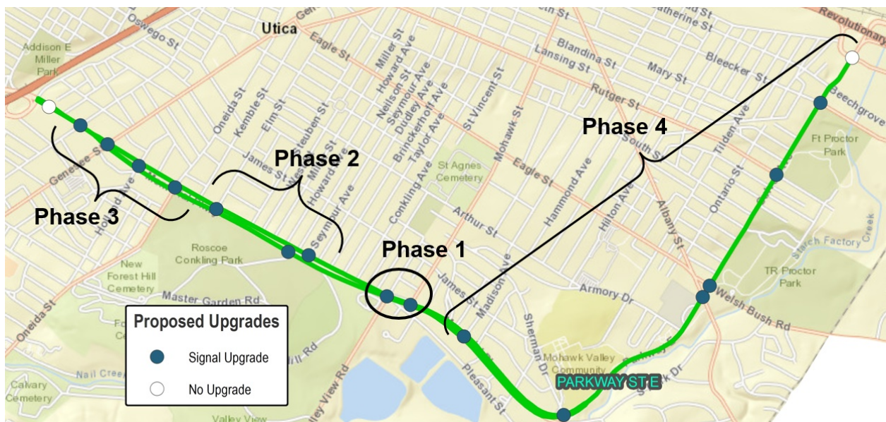
Figure 15. Proposed ITS Solutions for the Parkway Corridor
