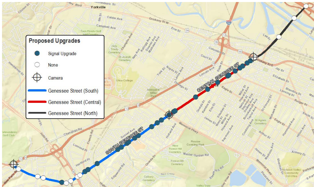
Figure 14. Proposed ITS Solutions for the Genesee Corridor
