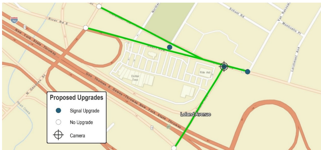
Figure 13. Leland Corridor Proposed ITS Layout
