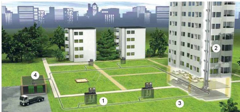
1 Exterior Inlets 2 Interior Inlets 3 Pipeline 4 Collection Terminal
