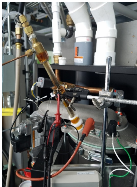
Figure 11. Residential Boiler Modified to Include Planar SOFC in Combustion Chamber
