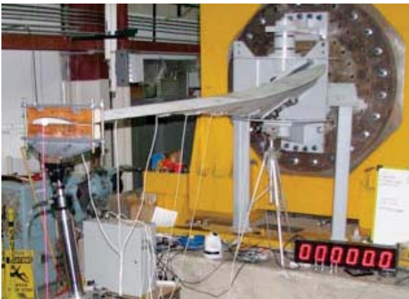
Fig. 8 – Gen 5a Rotor Assembly Testing Conducted at National Renewable Energy Laboratory
