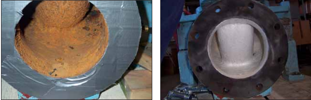
Figure 4.12 MCWA pump interior before (left) and after (right) sandblasting and coating
