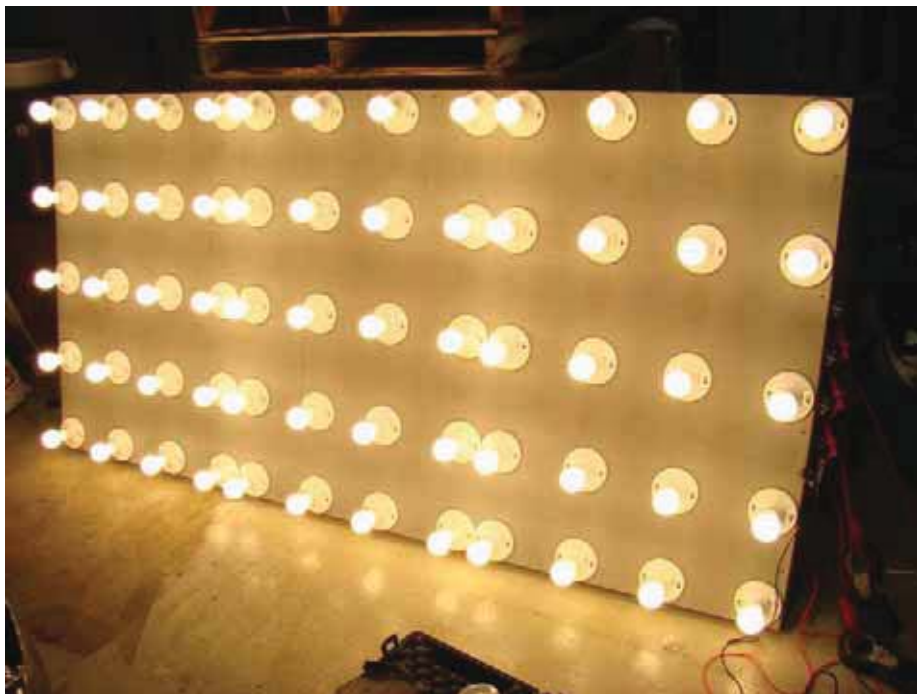
Figure 31 – Light Board used to generate harmonics
