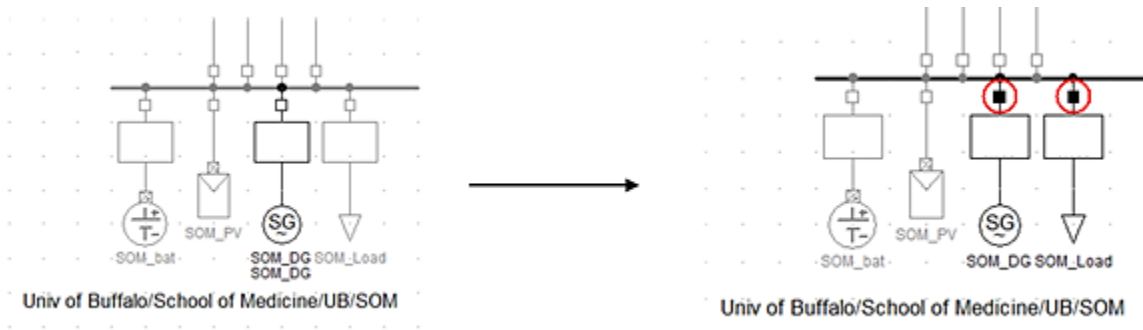
Figure 6-66 Black Start: Circuit condition
