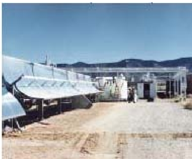
Figure 1-3. Single-axis parabolic-trough POC reactor developed by Sandia National Laboratory (1996). (Courtesy of National Renewable Energy Laboratory)
