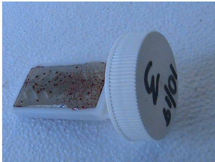
Figure 4-6. Dipslide indicating bacteria level after 1-hour of testing.
