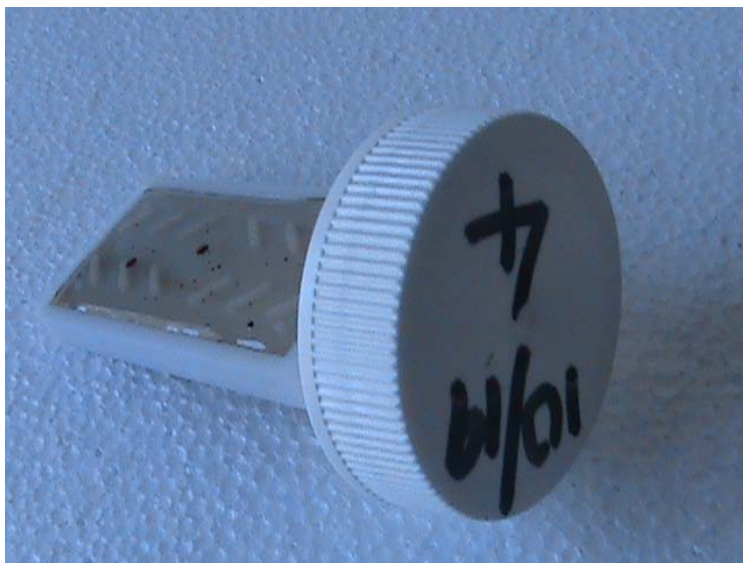
Figure 4-7. Dipslide indicating bacteria level after 2-hours of testing.
