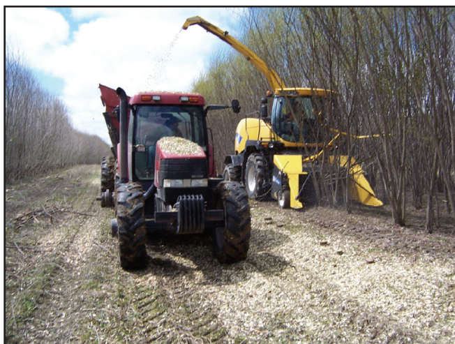
Figure 3ES: The NH 9060 Forage Harvester mounted with NH FR 130 SRWC header harvesting willow into a forage dump wagon in western NY.
