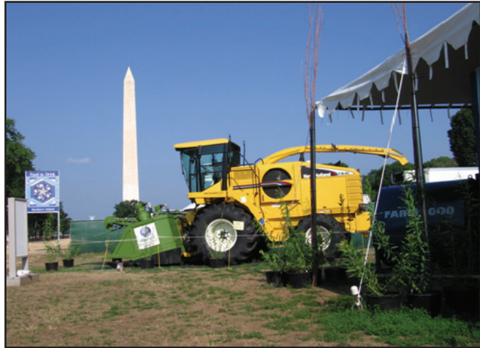
Figure 4ES: The single pass cut and chip harvesting system based on a New Holland forage harvester and modified CRL cutting head on display on the mall in Washington, DC
