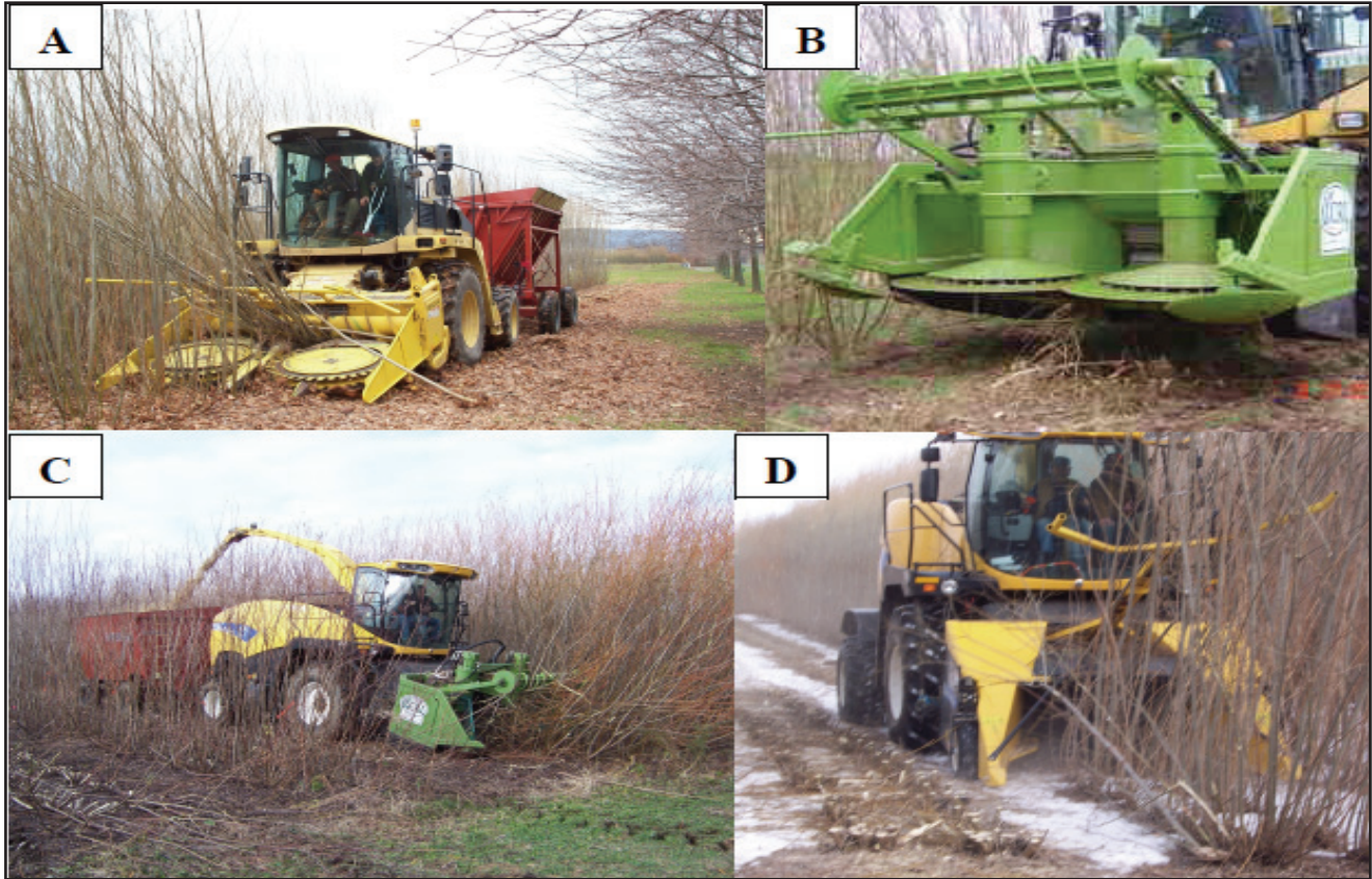
Figure 1ES: Development stages of the willow biomass harvesting system over the past few years in cooperation with Case New Holland. A-The FX series New Holland forage harvester with a modified corn head. B-The modified CRL willow cutting head mounted on a FX series New Holland forage harvester. C-The modified CRL willow cutting head mounted on the new FR series New Holland forage harvester. D-The newly designed New Holland short rotation coppice cutting head mounted on the FR series New Holland forage harvester.
