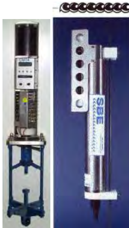
Figure 3-3 CM-04 Acoustic Current Meter (Left) and Seabird SBE37 CT Logger (Right)
