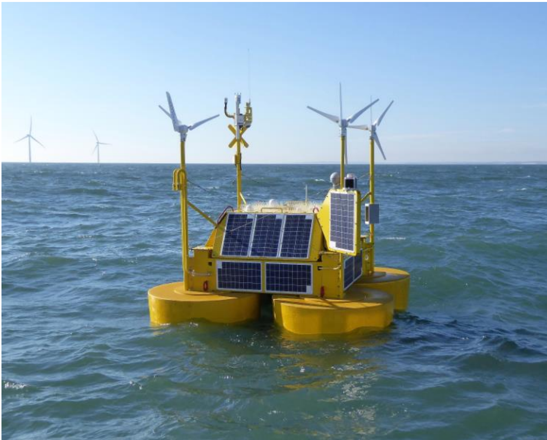
Figure 5-3 EOLOS FLS-200 buoy (DNV, 2022)
