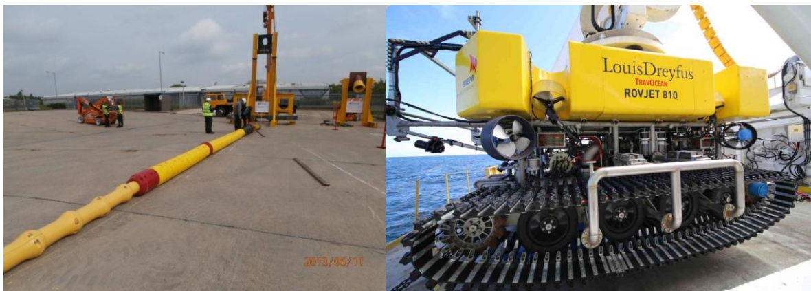
Figure 13-16 Example of a cable protection system test and cable trencher by RWE
