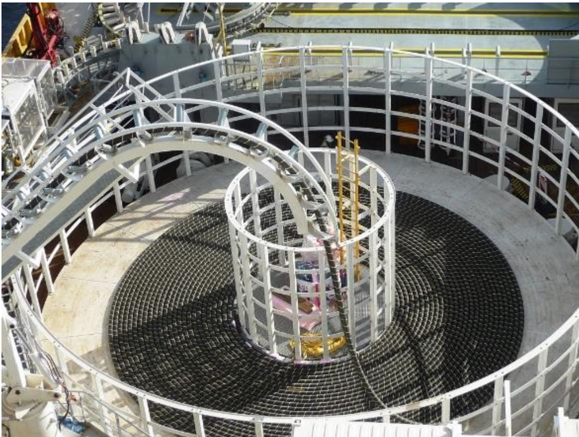
Figure 13-17 Example of inter-array cable storing by RWE
