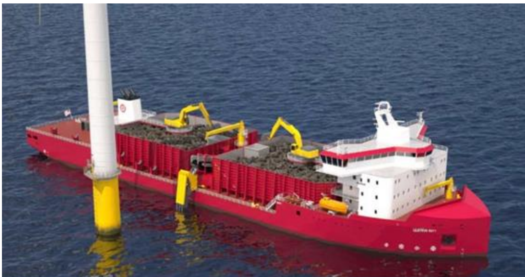
Figure 13-11 Fall pipe vessel example for scour protection installation
