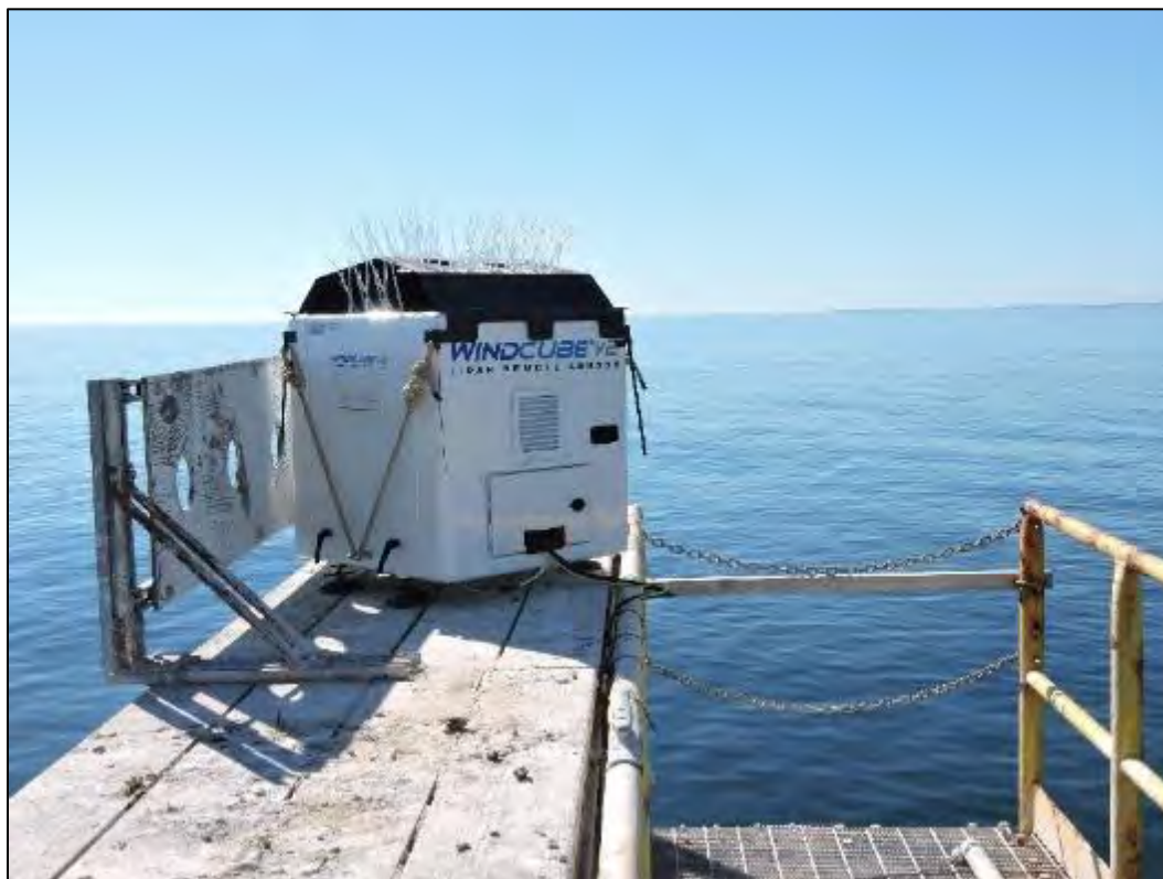
Figure 5.3 The WindCube V2 LiDAR located on the ASIT
