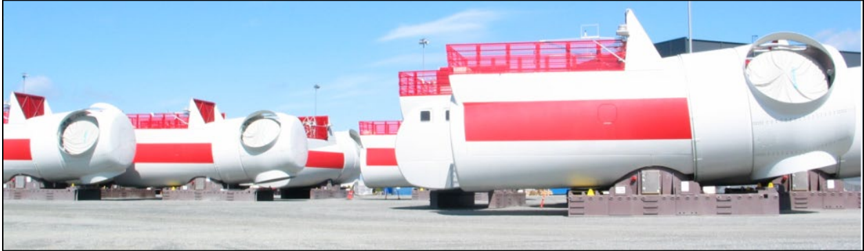
Figure 12.9 Nacelles Pre-assembled and Ready at the Load-out Port (Gode Wind, 2015)
