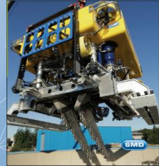
ROV in 'free-flying' mode For softer sediments where tracks would sink and cause a loss in maneuverability
