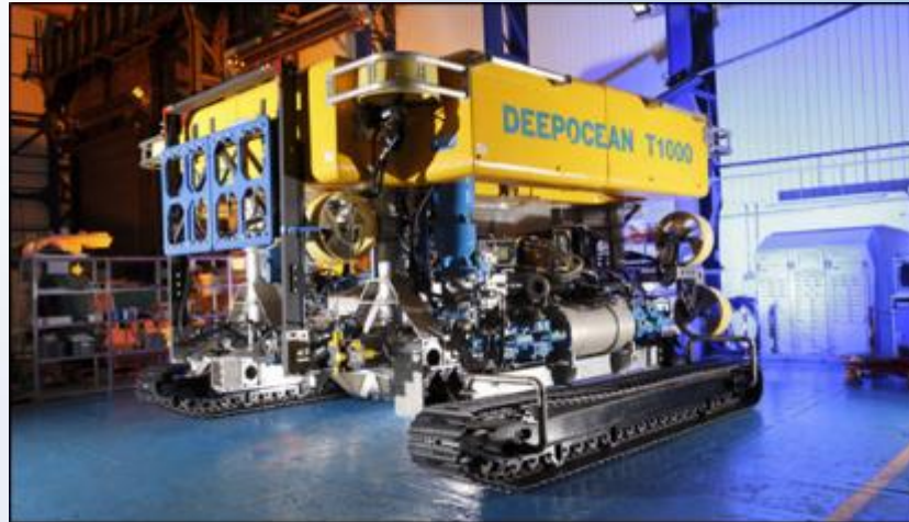
ROV Enshore's T1000 Up to 3m/10' burial depth Water jetting only
