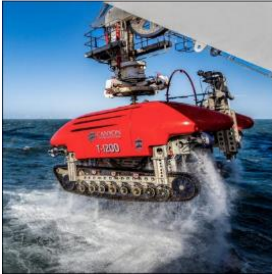
ROV Canyon's T1200 Up to 3m/10' burial depth Water jetting only
