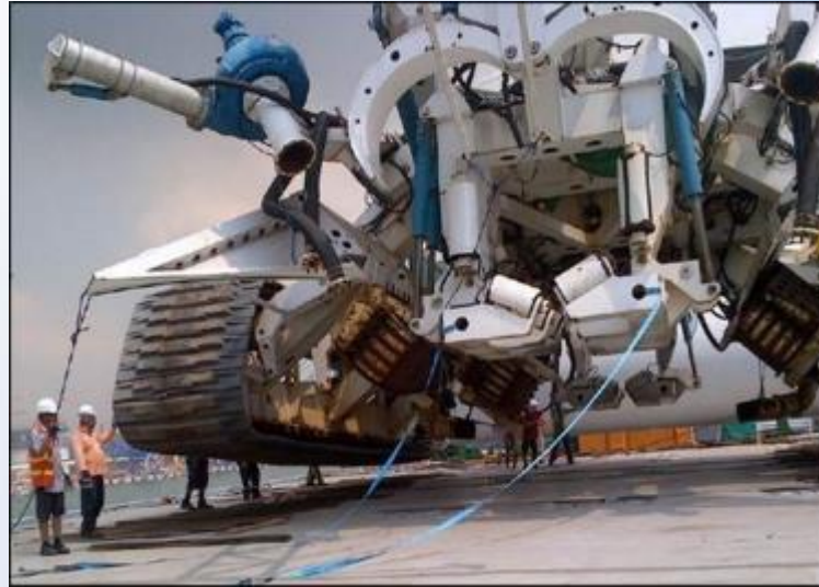
Tracked Trencher Deepoceans T3200 Weighs 170T, jetting and chain cutting up to 3.5m burial depth
