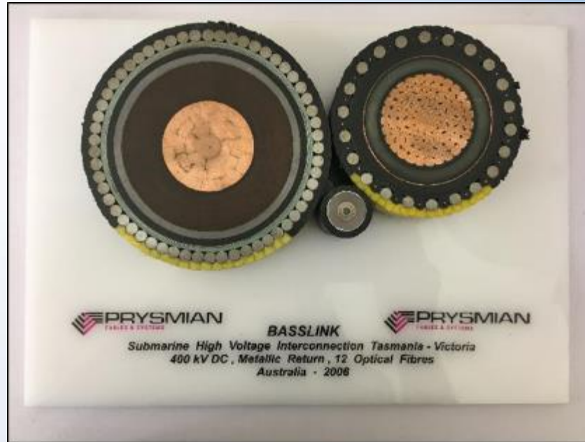
HVDC Cable 'slices' Neptune project on the left, Basslink (Tasmania) on the right
