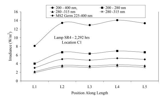
Figure 4.62 Integrated and germicidal irradiance of the aged Type 2 MP lamp SR4 as a function of position along the lamp length for location C1
