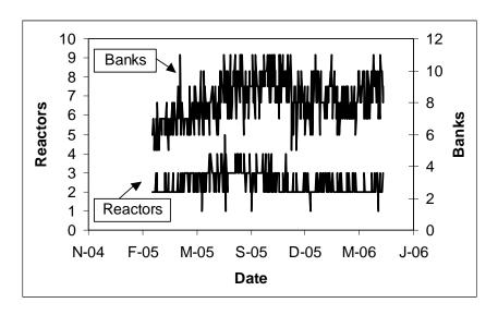
Figure 7.2 Number of operating reactor trains and banks per reactor predicted by the Advanced LCA UVCAT tool
