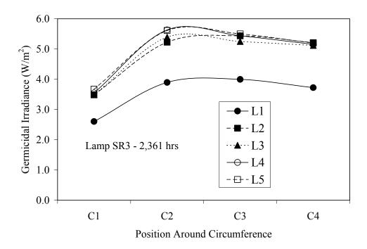
Figure 4.69 Germicidal irradiance of the aged Type 2 MP lamp SR3 as a function of position about the circumference
