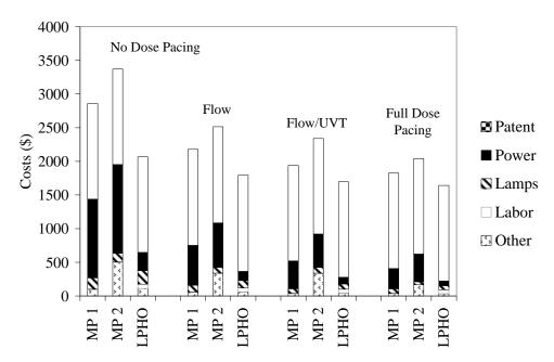
Figure 9.6 Impact of dose pacing strategies on O&M costs for the three hypothetical UV systems using lamp aging curves based on industry data; Electricity assumed \$0.05/kW-hr
