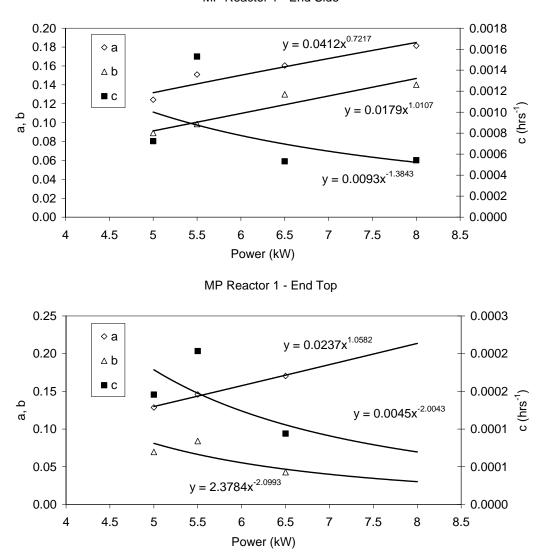
Figure 8.12 (Continued) Coefficients a, b, and c of Equation 8.1 plotted as a function of ballast power for the UV reactor equipped with four 8.0 kW MP lamps
