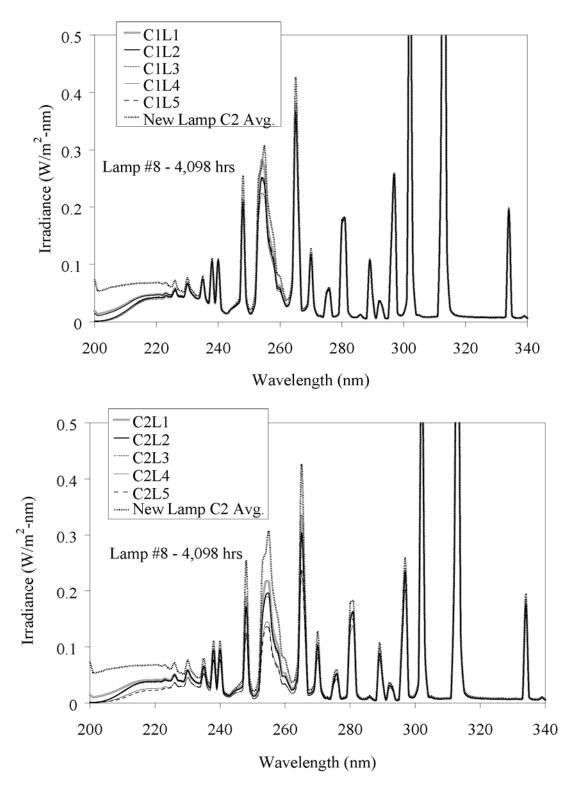
Figure 4.47 Spectral irradiance of Type 1 MP lamp #8 as a function of location along the lamp length and around the circumference (C1 - top, C2 - bottom)
