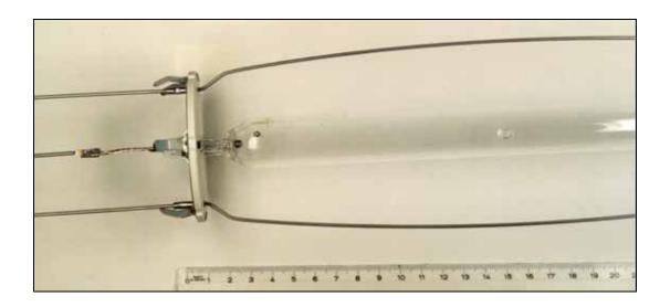
Figure 4.53 New Type 2 MP lamp
