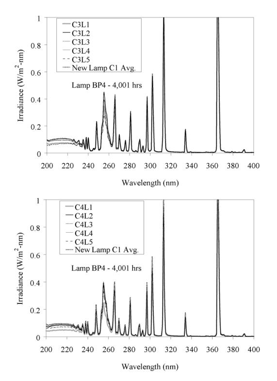
Figure 4.61 (Continued) Spectral irradiance of Type 2 MP lamp BP4 aged 4,001 hours as a function of location along the lamp length and around the circumference (C3 - top, C4 - bottom)
