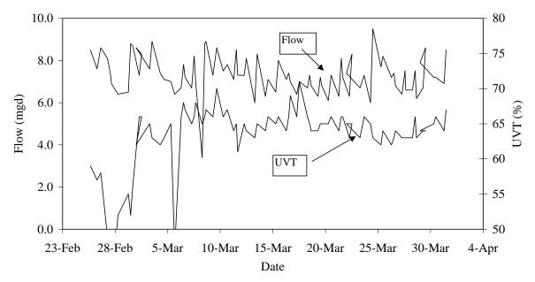
Figure 10.5 Flow rate and UVT at a California WWTP
