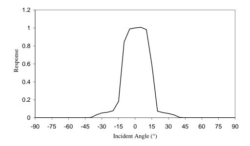
Figure 6.13 Angular response of DVGW and SiC UV sensors
