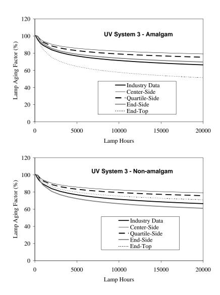
Figure 9.4 (Cont.) Lamp aging curves used in the UVCAT analysis of Lamp Aging Factors
