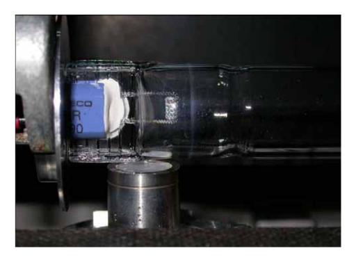
Figure 4.9 Location of SED 240 sensor relative to the lamp at the beginning of measurements of UV output along the length of the lamp
