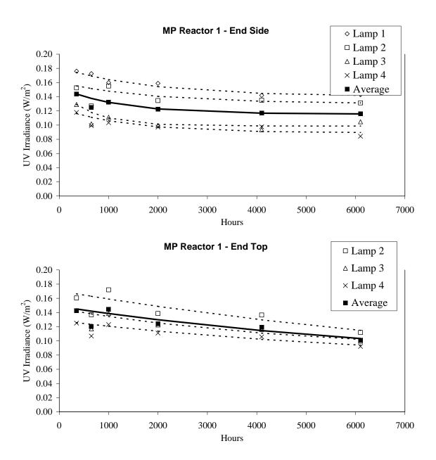
Figure 8.11 (Continued) Lamp aging data for the UV reactor equipped with four 8.0 kW MP lamps - Lamps 1, 2, 3, and 4 were operated at 8.0, 6.5, 5.5, and 5.0 kW, respectively
