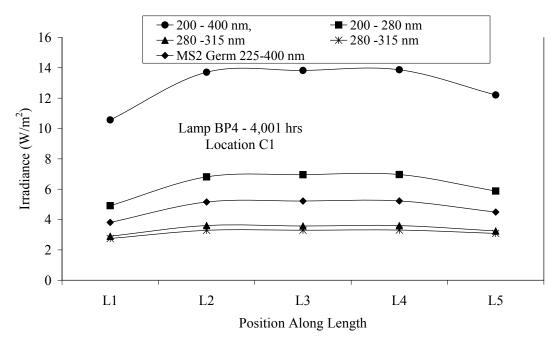
Figure 4.64 Integrated and germicidal irradiance of the aged Type 2 MP lamp BP4 as a function of position along the lamp length for location C1
