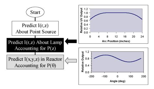
Figure 6.3 UV intensity algorithm accounts for non-uniform UV output along length and about the circumference of the lamp using weighting functions
