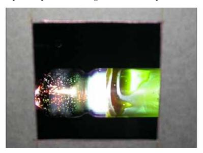
Figure 4.18 Unusual coloration of lamp #3 (6,188 hours) during operation, before it finally became defective (no color enhancement to photo)
