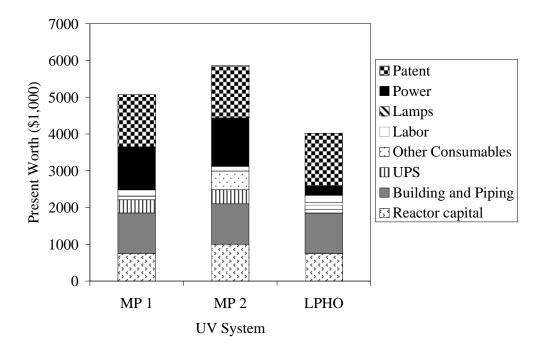
Figure 9.5 Present worth costs for the three hypothetical UV systems assuming no dose pacing and lamp aging curves based on industry data; Electricity assumed \$0.05/kW-hr
