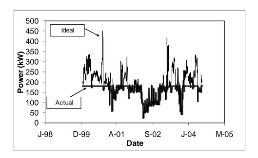
Figure 7.3 Power consumption by a UV system predicted by the Advanced LCA UVCAT tool under ideal and actual dose-pacing strategies
