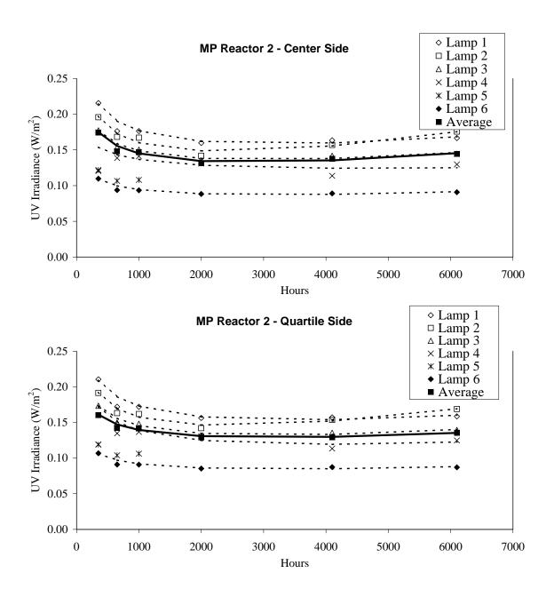
Figure 8.14 Lamp aging data for the UV reactor equipped with six 6.0-kW MP lamps - Lamps 1, 2, 3, 4, 5 and 6 were operated at 6.0, 6.0, 5.5, 5.0, 4.0, and 3.5 kW, respectively; Average excludes lamp 5
