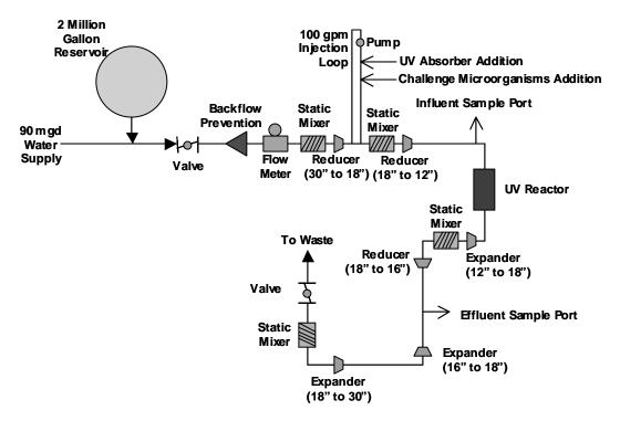
Figure 5.1 Test train schematic
