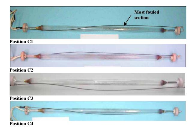
Figure 4.44 Photographs of the Type 1 MP lamp #8
