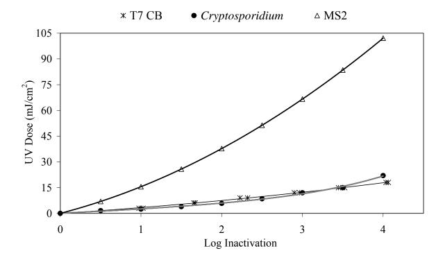
Figure 5.10 Comparison of MS2 and T7 UV dose-response with Cryptosporidium UV dose requirements
