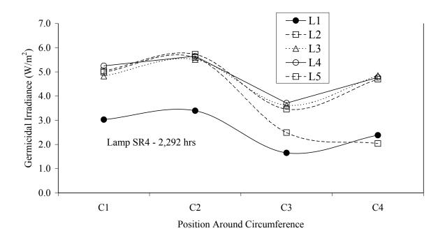
Figure 4.68 Germicidal irradiance of the aged Type 2 MP lamp SR4 as a function of position about the circumference
