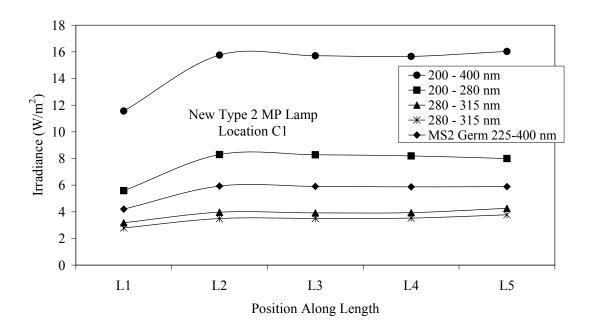
Figure 4.55 Integrated and germicidal irradiance of the new Type 2 MP lamp as a function of position along the lamp length for location C1
