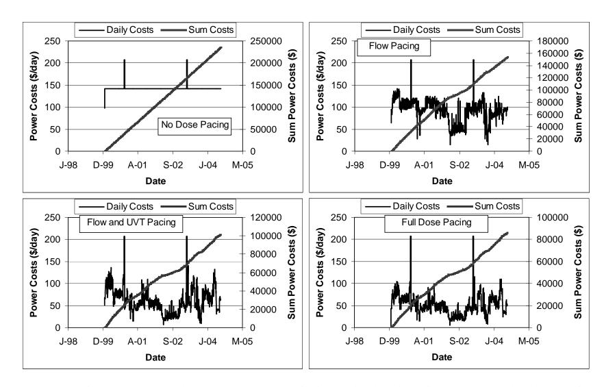
Figure 10.14 Case 3 power costs with no dose pacing (top left), flow pacing (top right), flow and UVT pacing (bottom left), and full dose pacing (bottom right)
