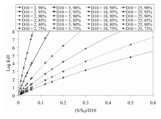
Figure 6.11 Log inactivation as a function of  $S/S_0/D_{10}$  and UVT for the LPHO reactor operating with 6 rows of lamps
