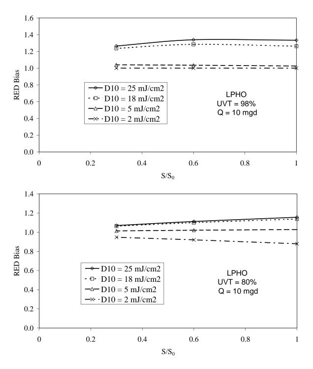
Figure 6.7 RED bias relative to  $D10=4~mJ/cm^2$  of the LPHO reactor with 6 rows of operating lamps as a function of relative lamp output  $(S/S_0)$  and microbe inactivation kinetics (D10) for 98 % UVT (top) and 80% UVT bottom
