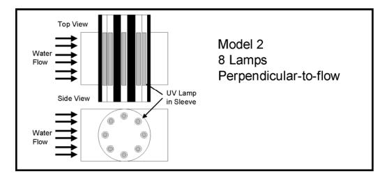
Figure 6.2 Schematic of the MP UV system
