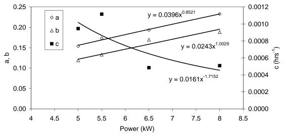
Figure 8.12 Coefficients a, b, and c of Equation 8.1 plotted as a function of ballast power for the UV reactor equipped with four  $8.0~\rm kW~MP$  lamps
