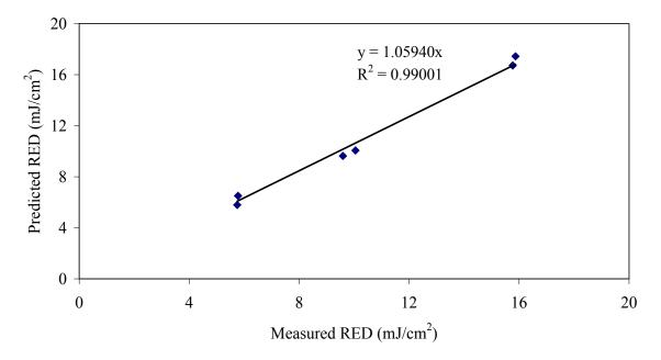
Figure 5.9 MS2 dose delivery predictions versus measured dose for MS2 field-testing conditions
