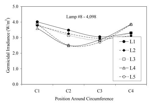
Figure 4.50 Germicidal irradiance of the aged Type 1 MP lamp #8 as a function of position about the circumference
