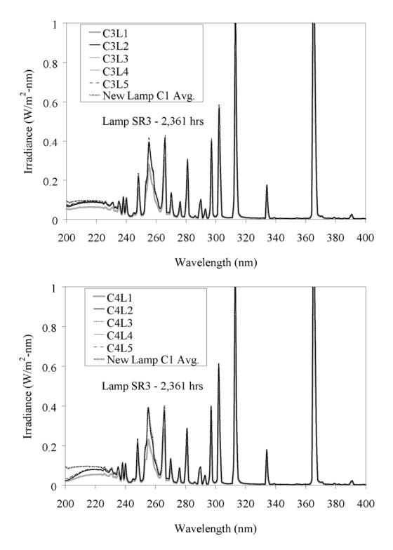
Figure 4.60 (Continued) Spectral irradiance of Type 2 MP lamp SR3 aged 2,361 hours as a function of location along the lamp length and around the circumference (C3 - top, C4 - bottom)
