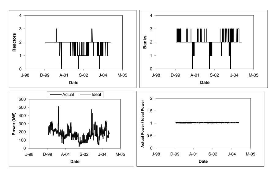
Figure 10.9 Case 1/three 3-bank reactors: reactors on (top left), banks on (top right), power consumption (bottom left), and ratio of ideal-to-actual power (bottom right)
