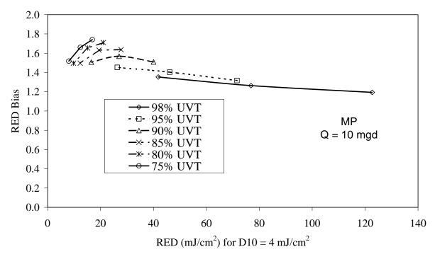
Figure 6.8 RED bias with the MP reactor as a function of RED based on D10 =  $4 \text{ mJ/cm}^2$ . RED bias is calculated as the ratio of REDs for D10 =  $18 \text{ and } 4 \text{ mJ/cm}^2$ .
