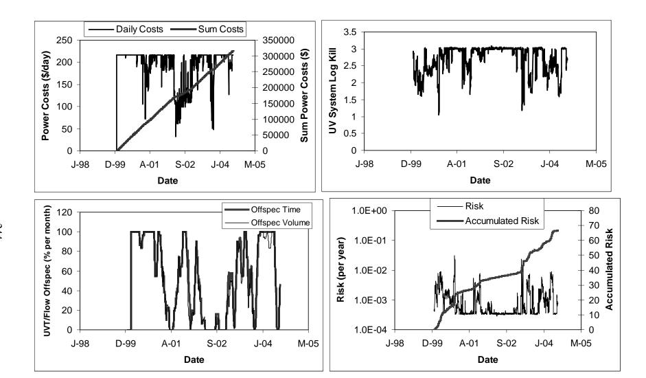
Figure 10.7 (Continued) Case 1/three 1-bank reactors: power costs (top left), UV system log kill (top right), off-specification performance (bottom left), health impact (bottom right)
