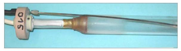
Figure 4.46 Close up of the coated end of Type 1 MP lamp #8 on the power supply side
