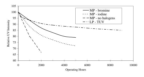
Figure 9.1 Lamp aging curves for LPHO and MP lamp technologies
