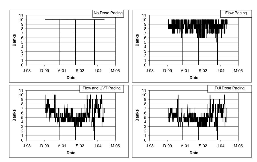
Figure 10.13 Case 3 banks operating over time with no dose pacing (top left), flow pacing (top right), flow and UVT pacing (bottom left), and full dose pacing (bottom right)
