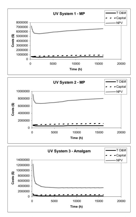
Figure 9.9 Impact of lamp replacement interval on life-cycle costs for the three hypothetical UV systems; Analysis uses lamp-aging curves from industry data, power costs of \$0.15/kW-hr, no dose pacing, and reactor capital costs varying with Lamp Aging Factor
