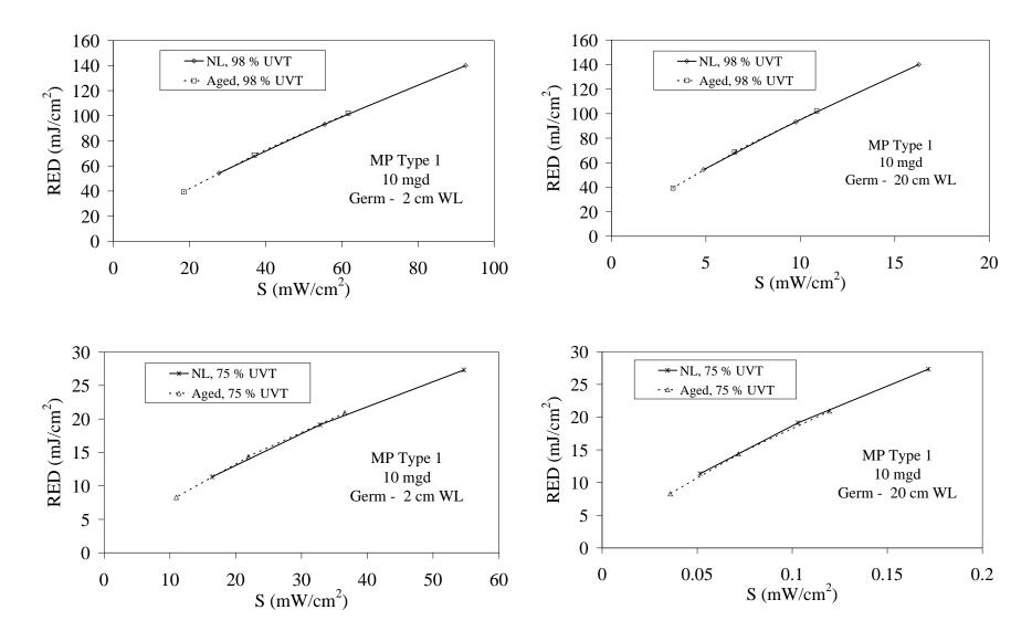
Figure 6.17 MS2 RED (D10 = 18 mJ/cm<sup>2</sup>) delivered by new and aged Type 1 MP lamps as a function of DVGW UV sensor readings for water layers of 2 and 20 cm and UVTs of 98 and 75%
