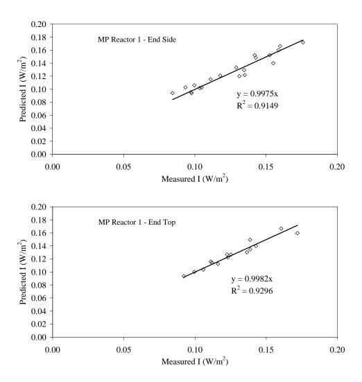
Figure 8.13 (Continued) Comparison of UV intensity predicted by Equation 8.2 to measured data
