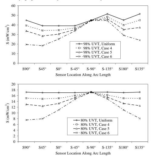
Figure 6.25 Impact of non-uniform MP lamp output about the circumference of the lamp on UV sensor readings (location  $S90^{\circ}$  -UV sensor views lamp #1 from above, location  $S^{\circ}0$  -UV sensor views lamp from the right hand side)
