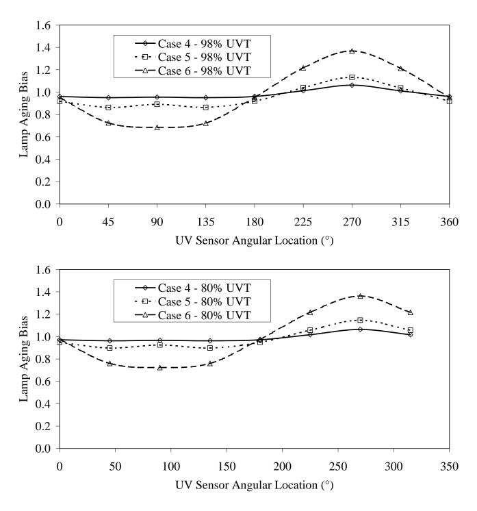
Figure 6.27 Dose monitoring bias caused by non-uniform lamp aging about the MP lamp's circumference as a function of angular UV sensor location ( $^{\circ}0$  - UV sensor views lamp from the right hand side,  $90^{\circ}$  - UV sensor views lamp from above)
