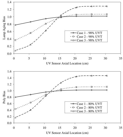
Figure 6.24 Dose monitoring bias caused by non-uniform MP lamp aging along the lamp length as a function of axial UV sensor location (0 cm - lamp end, 30 cm - lamp middle)
