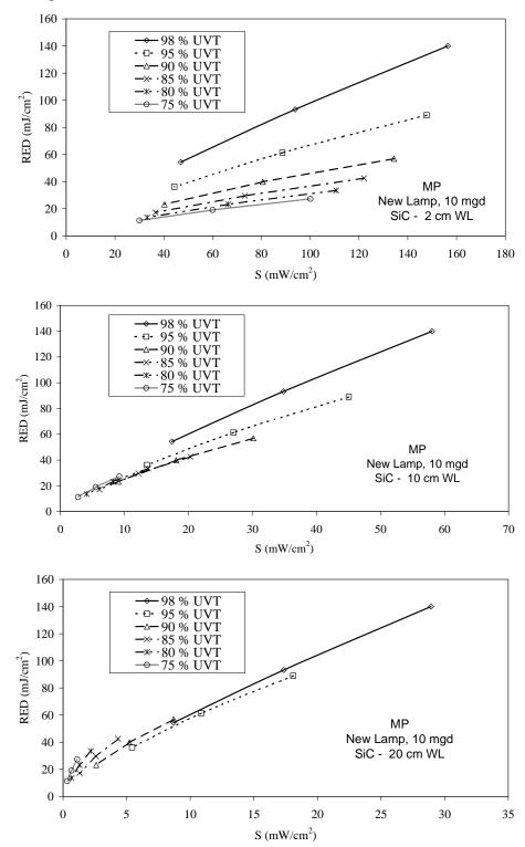
Figure 6.15 MS2 RED (D10 =  $18 \text{ mJ/cm}^2$ ) as a function of SiC UV sensor readings and UVT for water layers of 2, 10, and 20 cm
