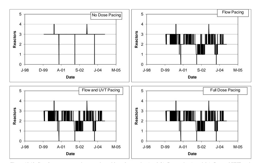
Figure 10.12 Case 3 reactors operating over time with no dose pacing (top left), flow pacing (top right), flow and UVT pacing (bottom left), and full dose pacing (bottom right)
