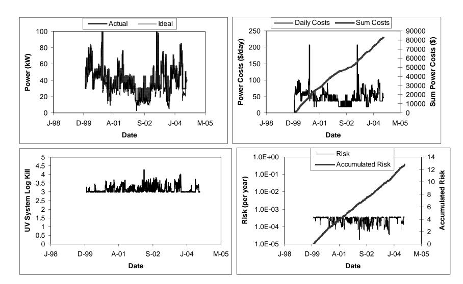
Figure 10.18 Case 4/1-bank UV system with full dose pacing: power consumption (top left), power costs (top right), UV system log kill (bottom left), health impact (bottom right)
