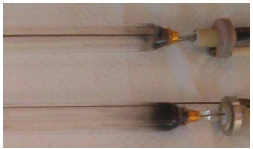
Figure 5.4 New lamp with 100-hour burnin (top) and the aged lamp (bottom) used duringfield-testing
