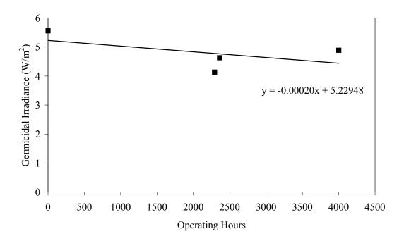
Figure 4.72 Germicidal irradiance as a function of operating hours with Type 2 MP lamps
