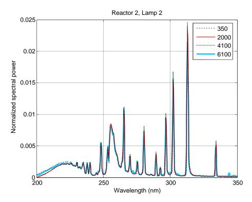
Figure 8.16 Spectral irradiance for medium pressure lamp #2, reactor #2 recorded at different operating times over the course of the study
