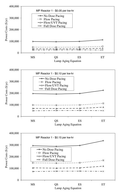
Figure 9.7 Impact of power costs and dose pacing strategies on O&M costs for UV System 1 using lamp aging curves based on MP lamp aging data measured in this project
