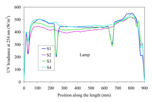
Figure 4.31 UV output at 254 nm of LPHO lamp #8 (1,472 hours) as a function of position along the length and around the circumference
