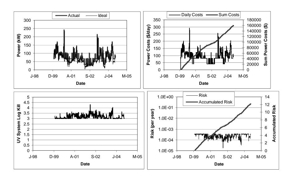
Figure 10.10 Case 2/four-train UV system with electronic ballasts: power consumption (top left), power costs (top right), log inactivation (bottom left), public health protection (bottom right)
