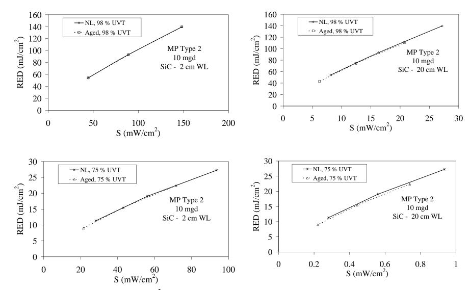
Figure 6.18 MS2 RED (D10 = 18 mJ/cm<sup>2</sup>) delivered by new and aged Type 2 MP lamps as a function of SiC UV sensor readings for water layers of 2 and 20 cm and UVTs of 98 and 75%
