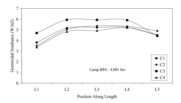
Figure 4.67 Germicidal irradiance of the aged Type 2 MP lamp BP4 as a function of position along the lamp length
