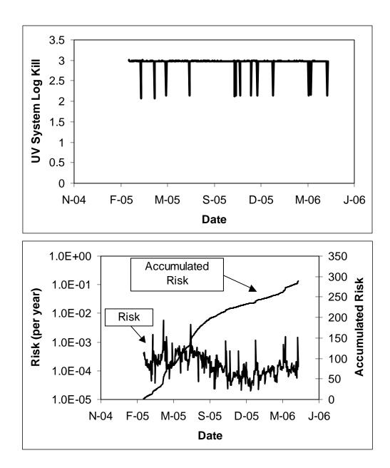
Figure 12.12 UV system log inactivation (top), and annual infection risk and accumulated infection (bottom) for the Case 3 LPHO system
