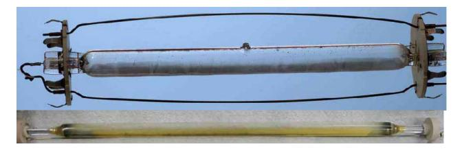
Figure 4.12 Discoloration along lamp length but around only  $180^{\circ}$  of the circumference
