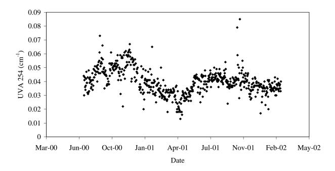
Figure 10.1 Poughkeepsie WTP filter effluent UV absorbance
