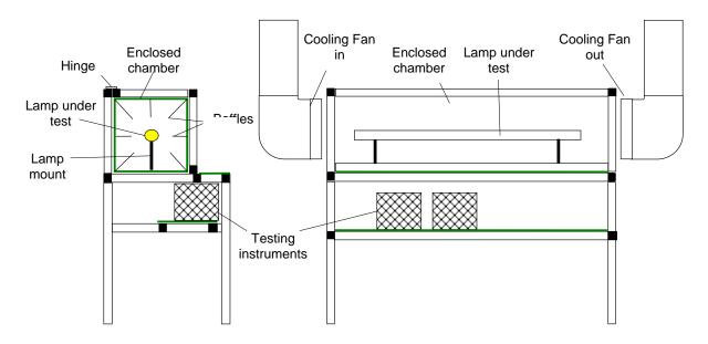
Figure 8.6 Schematic of the measurement chamber
