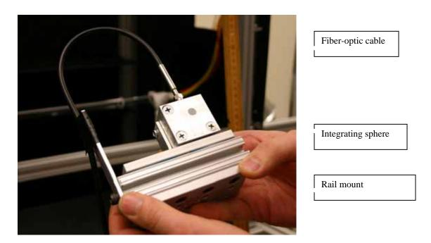
Figure 8.9 Input optics to the fiber-coupled monochromator. Integrating sphere optics provided cosine response for proper irradiance measurements.
