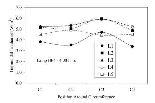
Figure 4.70 Germicidal irradiance of the aged Type 2 MP lamp BP4 as a function of position about the circumference
