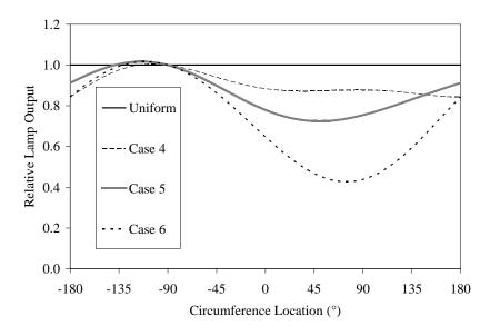
Figure 6.20 UV output about the circumference of the lamp used in the MP system analysis
