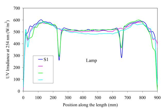
Figure 4.29 UV output at 254 nm of LPHO lamp #1 (940 hours) as a function of position along the length and around the circumference of the lamp
