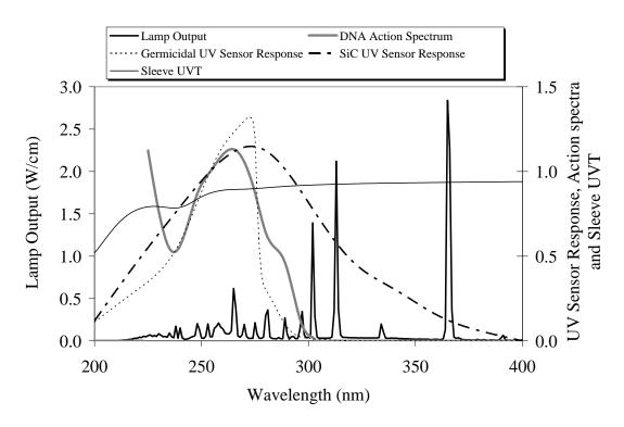
Figure 3.8 Lamp output, UV sensor spectral response, and microbial action data used as inputs to the Polychromatic Bias worksheet
