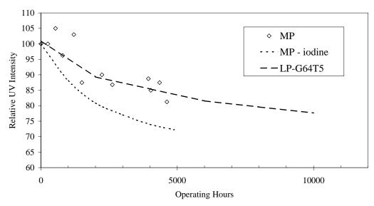
Figure 9.2 Lamp aging data for three lamp types
