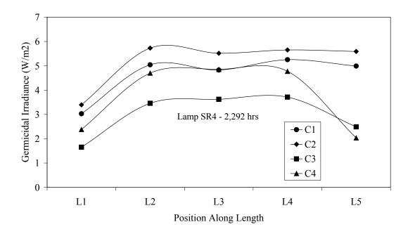
Figure 4.65 Germicidal irradiance of the aged Type 2 MP lamp SR4 as a function of position along the lamp length
