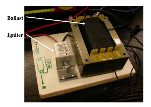
Figure 4.3 LPHO ballast and igniter
