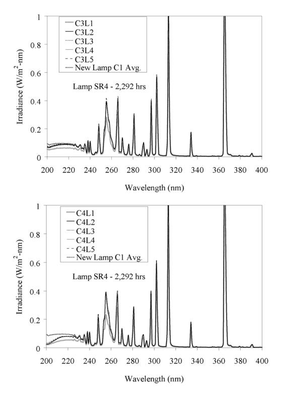
Figure 4.59 (Continued) Spectral irradiance of Type 2 MP lamp SR4 aged 2,292 hours as a function of location along the lamp length and around the circumference (C3 - top, C4 - bottom)
