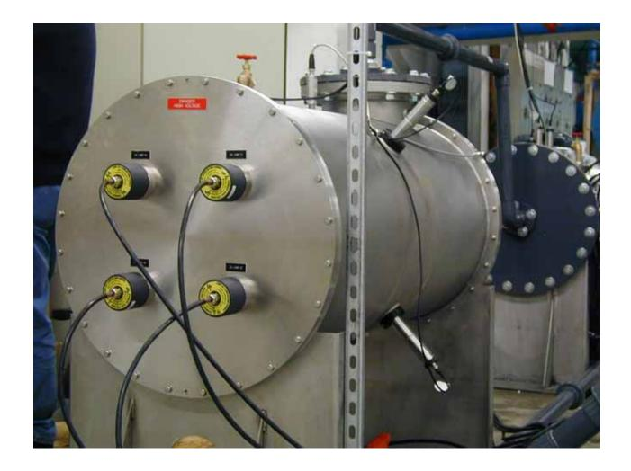
Figure 8.4 Photograph of the IDI reactor equipped with four 4 kW MP lamps
