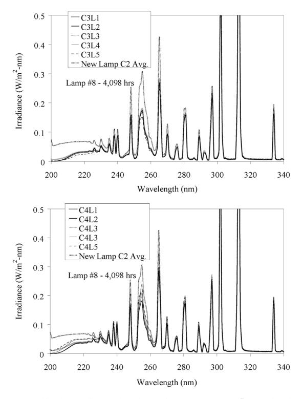
Figure 4.47 (Continued) Spectral irradiance of Type 1 MP lamp #8 as a function of location along the lamp length and around the circumference (C3 - top, C4 - bottom)
