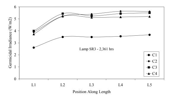
Figure 4.66 Germicidal irradiance of the aged Type 2 MP lamp SR3 as a function of position along the lamp length
