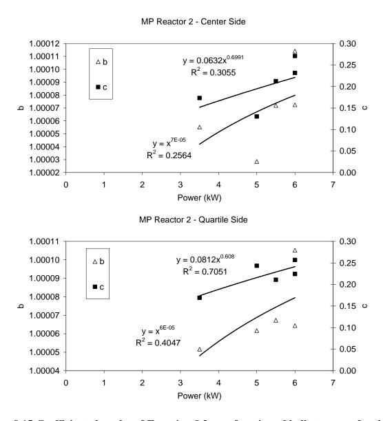
Figure 8.15 Coefficients b and c of Equation 8.3 as a function of ballast power for the UV reactor equipped with six 6.0-kW MP lamps
