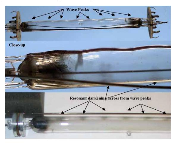
Figure 4.15 Resonant distortion and darkening with a MP lamp
