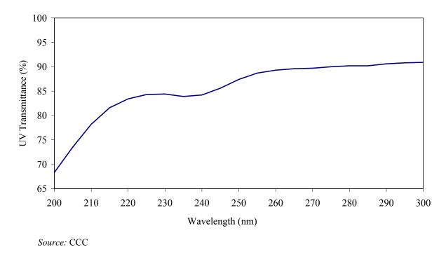
Figure 5.3 UV transmittance of a 1.5 mm thick lamp sleeve for a  $90^{\circ}$  of incidence angle and air-quartz interfaces
