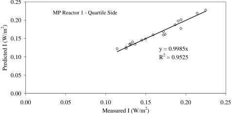
Figure 8.13 Comparison of UV irradiance predicted by Equation 8.2 to measured data
