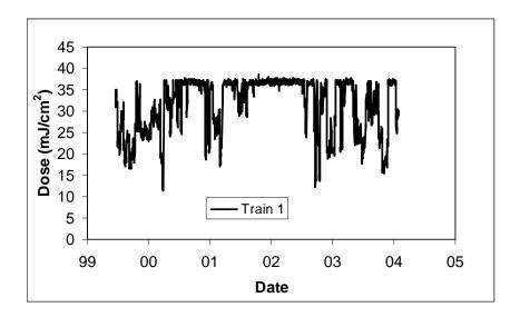
Figure 7.8 UV dose delivery over time predicted by the Advanced LCA UVCAT tool
