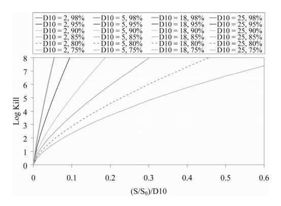
Figure 6.10 Log inactivation as a function of S/S<sub>0</sub>/D<sub>10</sub> and UVT for the MP reactor
