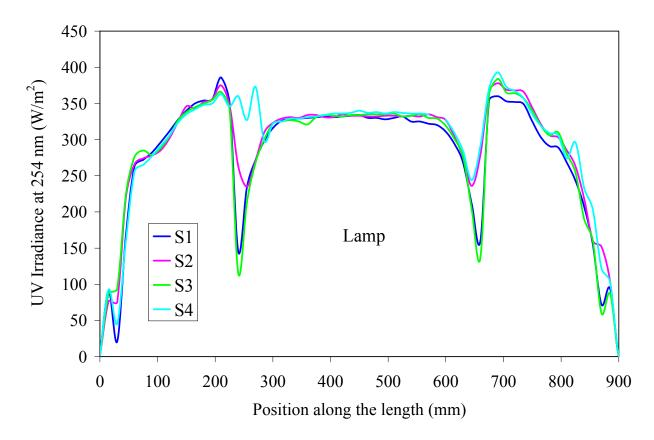
Figure 4.33 UV output at 254 nm of LPHO lamp #9 (6,696 hours) as a function of position along the length and around the circumference
