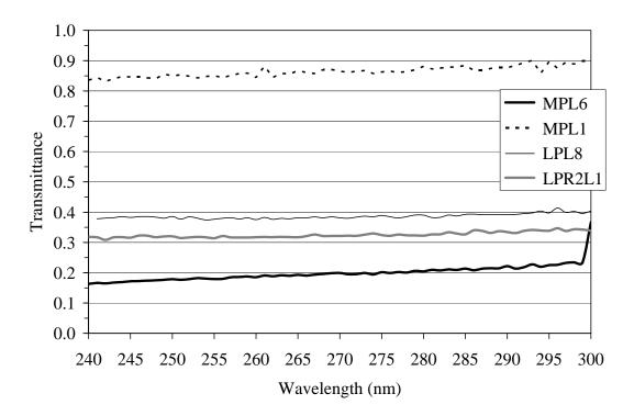
Figure 8.20 UV transmittance of quartz sleeve samples taken from the medium pressure reactors (MP) and the LPHO reactors (LP). The transmittance curves shown are the average of three samples
