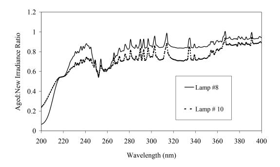
Figure 4.51 Ratio of UV irradiance measured with old Type 1 MP lamps to that measured with new lamps as a function of wavelength
