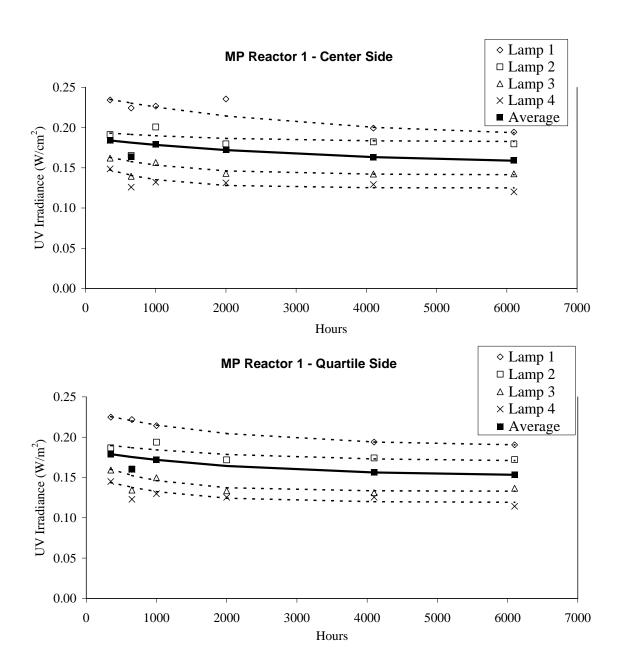
Figure 8.11 Lamp aging data for the UV reactor equipped with four 8.0 kW MP lamps - Lamps 1, 2, 3, and 4 were operated at 8.0, 6.5, 5.5, and 5.0 kW, respectively
