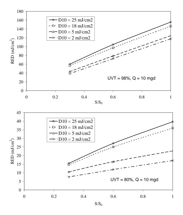
Figure 6.4 RED delivered by the MP reactor as a function of relative lamp output ( $S/S_0$ ) and microbe inactivation kinetics (D10) for 98 % UVT (top) and 80% UVT bottom
