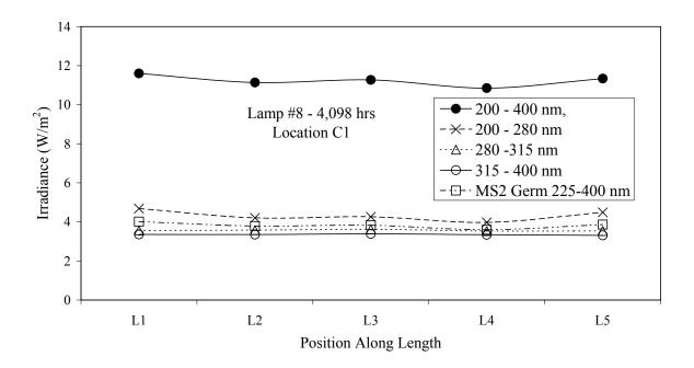
Figure 4.48 Integrated and germicidal irradiance of the aged Type 1 MP lamp #8 as a function of position along the lamp length at location C1
