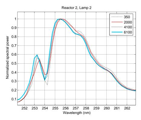
Figure 8.17 Expanded wavelength axis (zoom) of Figure 8.16 in the wavelength vicinity of the principle Hg emission line at 254 nm
