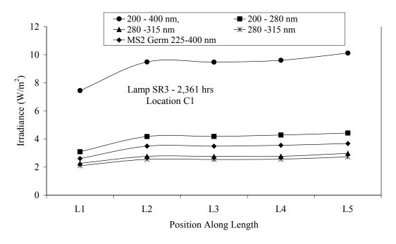
Figure 4.63 Integrated and germicidal irradiance of the aged Type 2 MP lamp SR3 as a function of position along the lamp length for location C1
