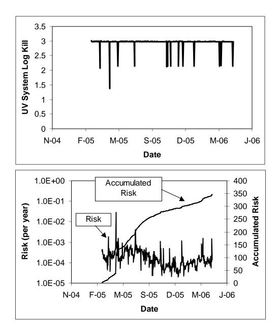
Figure 12.11 UV system log inactivation (top), and annual infection risk, and accumulated infection for the Case 2 LPHO system (bottom)
