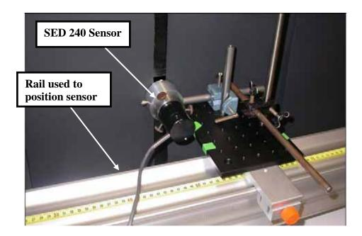
Figure 4.7 Mounting of SED 240 sensor used to measure UV lamp output at 254 nm along length of lamp
