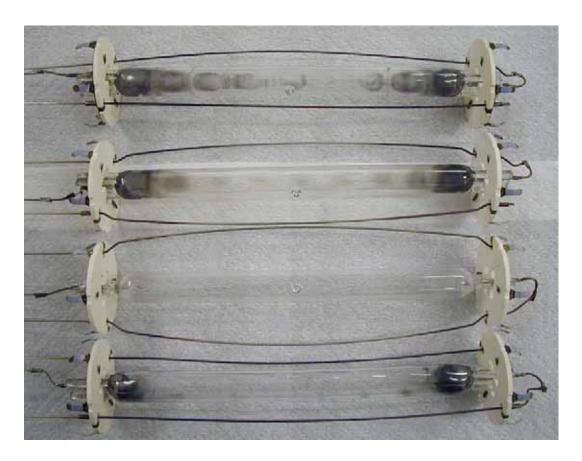
Figure 4.1 Discoloration observed with aged MP lamps after approximately 4000 hours of operation compared to a relatively new lamp (third down from top)
