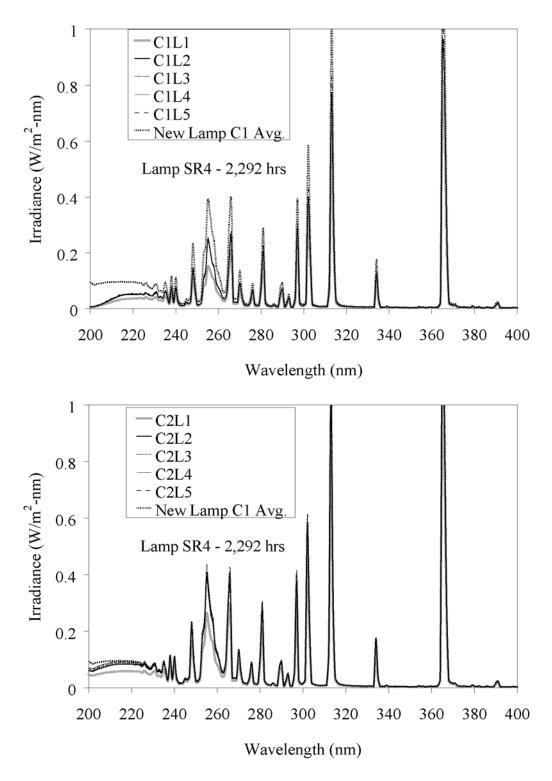
Figure 4.59 Spectral irradiance of Type 2 MP lamp SR4 aged 2,292 hours as a function of location along the lamp length and around the circumference (C1 - top, C2 - bottom)
