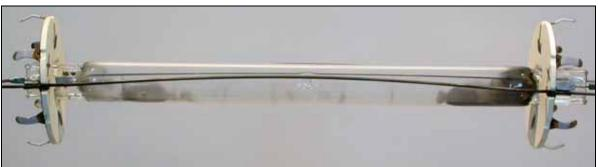
Figure 4.56 Type 2 MP lamp aged 2,292 hours (SR4) photographed from location C2 (top) and C3 (bottom)
