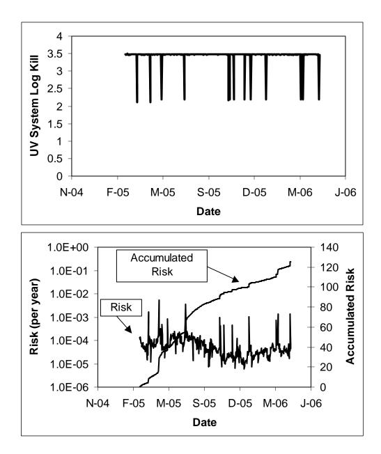
Figure 12.15 UV system log inactivation (top), and annual infection risk and accumulated infection (bottom) for the Case 6 LPHO system
