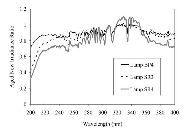
Figure 4.71 Ratio of UV irradiance measured with old Type 2 MP lamps to that measured with new lamps as a function of wavelength
