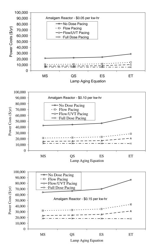
Figure 9.8 Impact of power costs and dose pacing strategies on O&M costs for UV System 3 using lamp aging curves based on amalgam lamp aging data measured in this project
