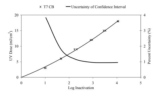
Figure 5.8 UV dose-response of T7 phage measured during testing
