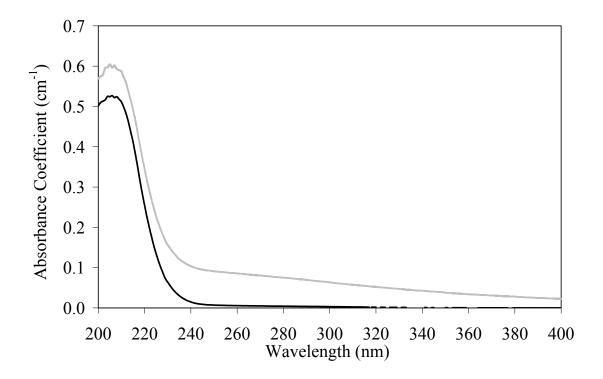
Figure 5.5 Spectral UV absorbance coefficients of raw test water and test water with Super  $Hume^{TM}$
