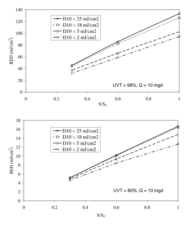
Figure 6.5 RED delivered by the 6-row LPHO reactor as a function of relative lamp output  $(S/S_0)$  and microbe inactivation kinetics (D10) for 98 % UVT (top) and 80% UVT bottom
