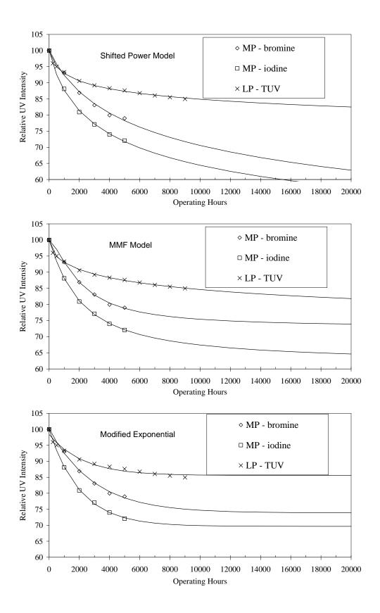
Figure 9.3 (Cont.) Model fits (curves) to lamp aging data (symbols)
