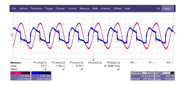
Figure 8.22 Oscilloscope traces of lamp current (C2, pink trace) and electrode heating voltage (C3, blue trace) for a stable operating lamp
