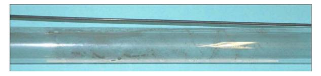
Figure 4.45 Close up on the most fouled section of Type 1 MP lamp #8 (Position C1)
