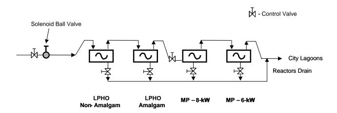
Figure 8.1 Schematic of the test process train installed at the John P. Buckley WTP
