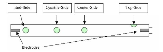
**Figure 8.5 Spectral measurement positions**
