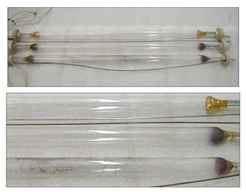
Figure 4.35 Type 1 MP lamps analyzed: full view (top photo) and close-up (bottom photo). Lamp ages are, from top to bottom: 0, 3,266, and 4,098 hours, respectively
