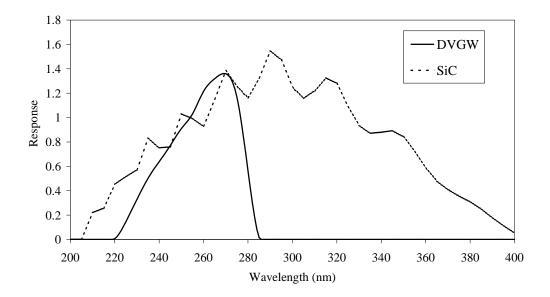
Figure 6.12 Spectral response of DVGW and SiC UV sensors
