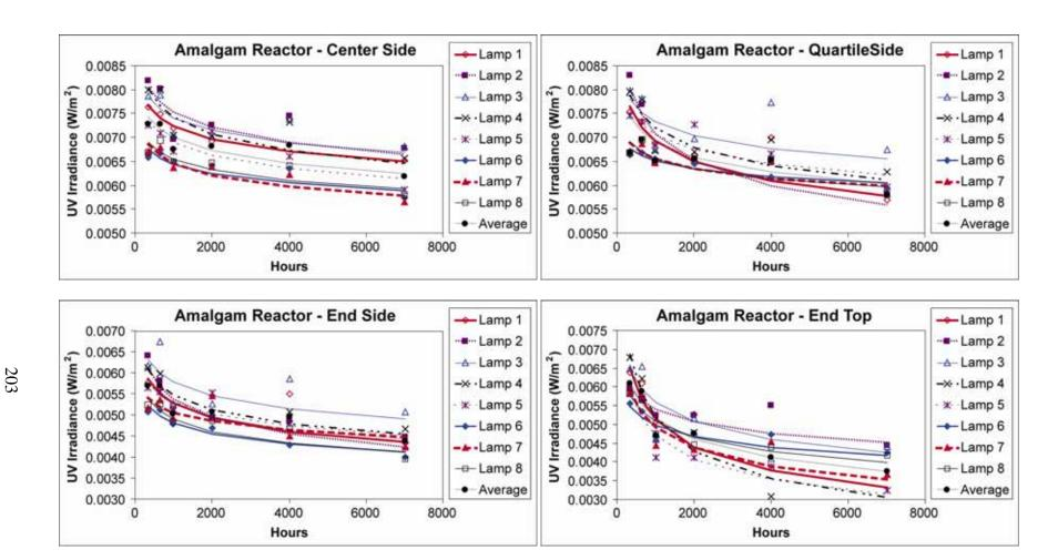
Figure 8.18 Lamp aging data for the UV reactor equipped with eight 300-W amalgam LPHO lamps. Lamps 1 through 4 operated at 100% power; Lamps 5 through 8 operated at 80% power
