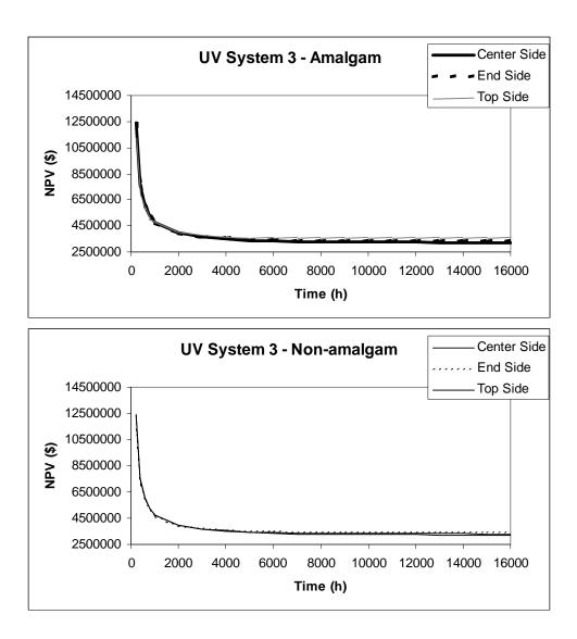
Figure 9.10 (Continued) Impact of lamp replacement interval on life-cycle costs for the modeled UV systems, Analysis uses lamp-aging curves from data measured in this project, power costs of \$0.15/kW-hr, no dose pacing, and reactor capital costs varying with Lamp Aging Factor
