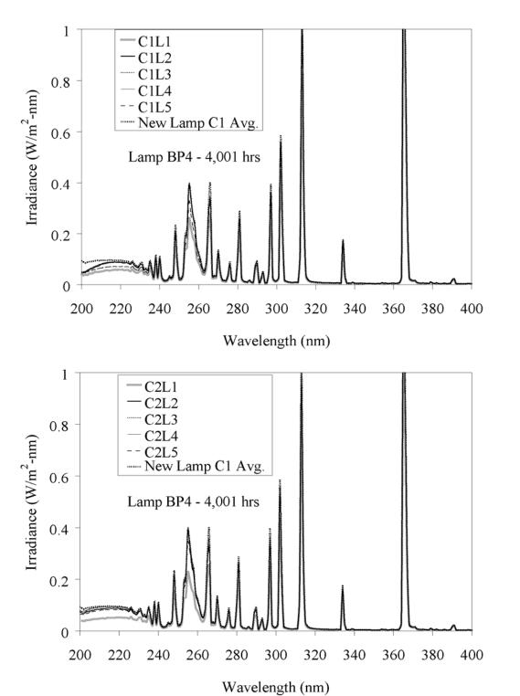
Figure 4.61 Spectral irradiance of Type 2 MP lamp BP4 aged 4,001 hours as a function of location along the lamp length and around the circumference (C1 - top, C2 - bottom)
