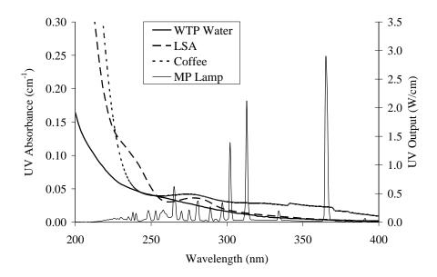
Figure 3.1 UV output of an MP lamp and absorbance spectra of a natural WTP water and UVA surrogates commonly used during UV reactor validation (coffee and LSA)
