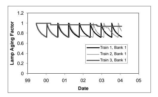
Figure 7.5 Lamp-aging simulated by the Advanced LCA UVCAT tool
