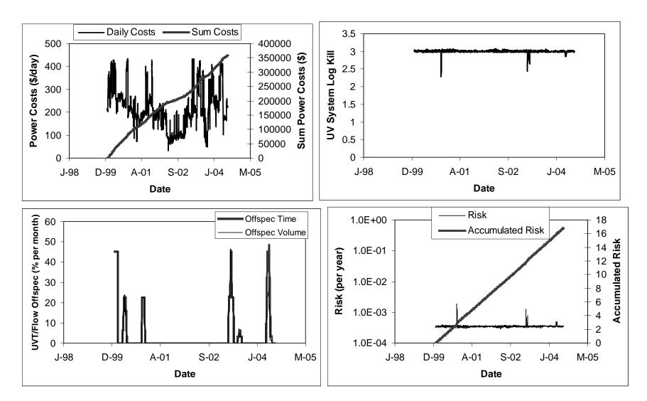
Figure 10.8 (Continued) Case 1/three 2-bank reactors: power costs (top left), UV system log kill (top right), off-specification performance (bottom left), health impact (bottom right)
