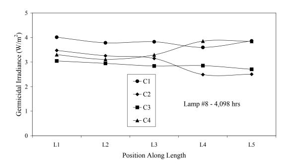
Figure 4.49 Germicidal irradiance of the aged Type 1 MP lamp #8 as a function of position along the lamp length
