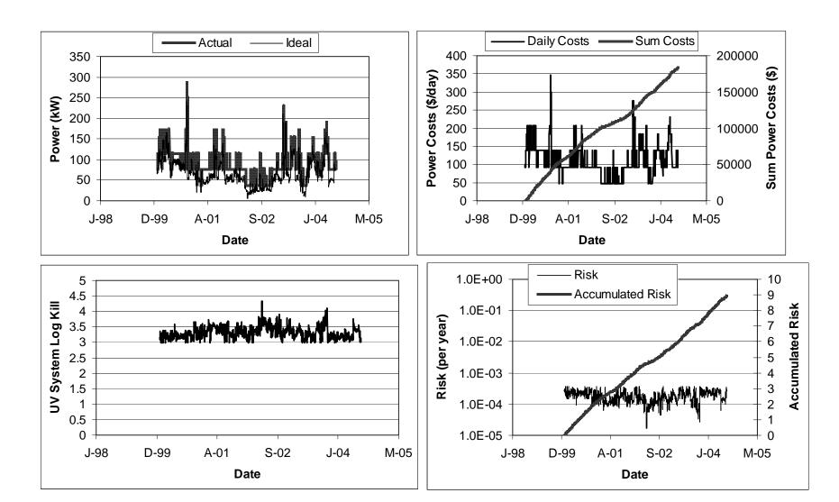
Figure 10.11 Case 2/four-train UV system with electromagnetic ballasts: power consumption (top left), power costs (top right), log inactivation (bottom left), public health protection (bottom right)
