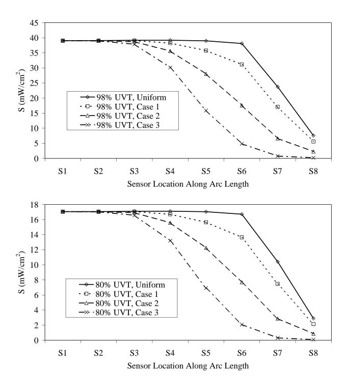
Figure 6.22 Impact of non-uniform MP lamp output along the lamp length on UV sensor readings (location S1 - center of the lamp, location S7 - lamp end, spacing between UV sensors -  $5~\rm cm$ )
