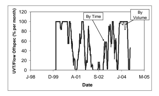
Figure 7.7 Off-specification performance over time predicted by the Advanced LCA UVCAT tool
