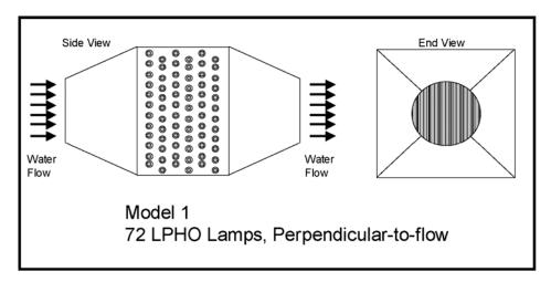
Figure 6.1 Schematic of the LPHO UV system
