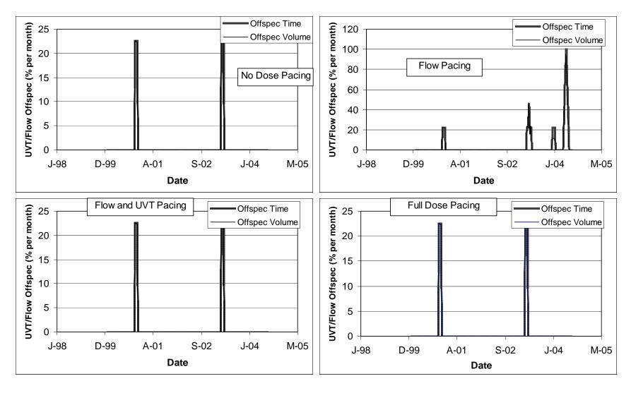
Figure 10.15 Case 3 off spec performance with no dose pacing (top left), flow pacing (top right), flow and UVT pacing (bottom left), and full dose pacing (bottom right)
