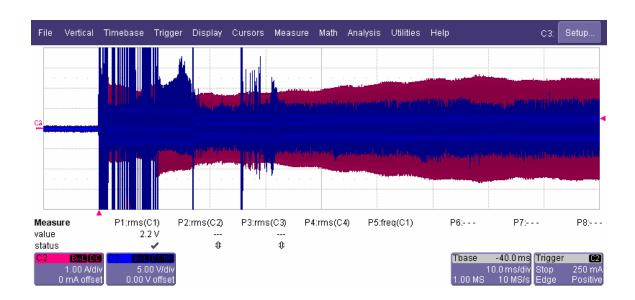
Figure 8.23 Oscilloscope traces of lamp current (C2, pink trace) and electrode heating voltage (C3, blue trace) during the starting of the lamp
