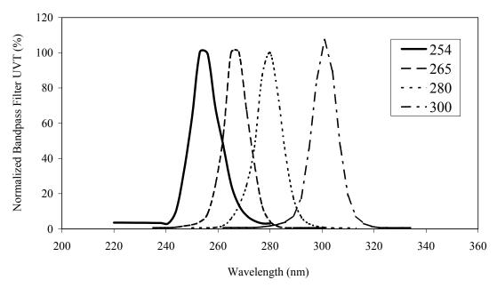
Figure 2.1 T4 bandpass filter UV transmittance
