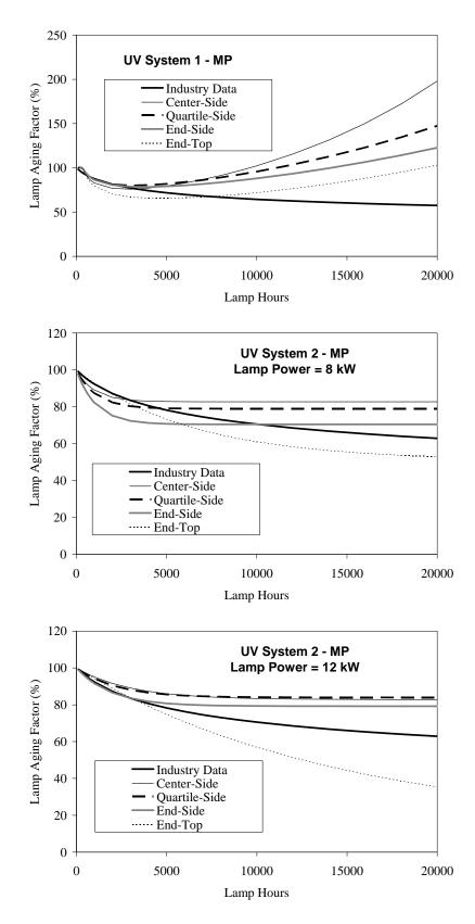
Figure 9.4 Lamp aging curves used in the UVCAT analysis of Lamp Aging Factors
