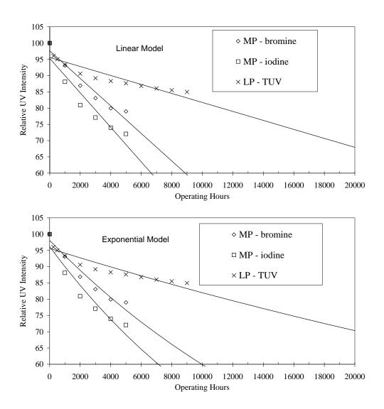
Figure 9.3 Model fits (curves) to lamp aging data (symbols)
