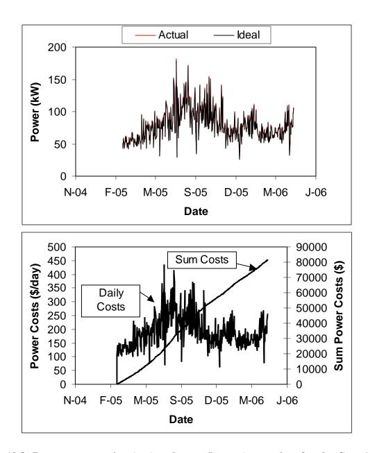
Figure 12.8 Power consumption (top) and costs (bottom) over time for the Case 1 LPHO system  $\frac{1}{2}$
