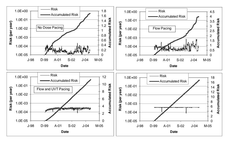
Figure 10.17 Case 3 public health protection with no dose pacing (top left), flow pacing (top right), flow and UVT pacing (bottom left), and full dose pacing (bottom right)
