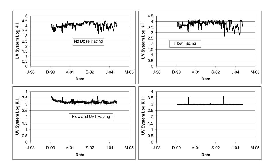
Figure 10.16 Case 3 *Cryptosporidium* inactivation with no dose pacing (top left), flow pacing (top right), flow and UVT pacing (bottom left), and full dose pacing (bottom right)
