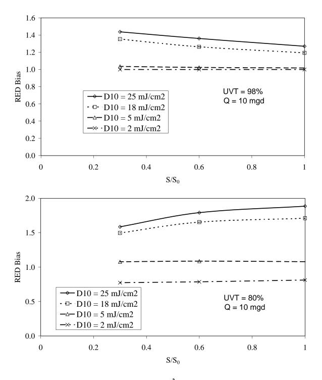
Figure 6.6 RED bias relative to  $D10=4~mJ/cm^2$  of the MP reactor as a function of relative lamp output (S/S<sub>0</sub>) and microbe inactivation kinetics (D10) for 98 % UVT (top) and 80% UVT bottom
