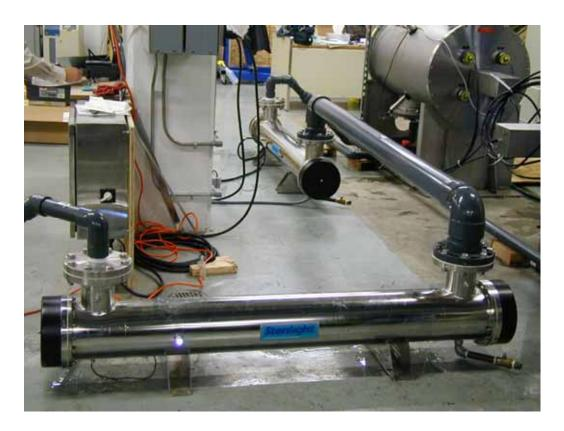
Figure 8.2 Photograph of the R-Can amalgam and non-amalgam LPHO reactors
