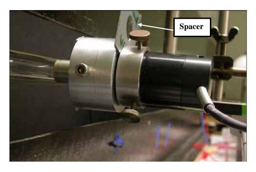
Figure 4.8 SED 240 sensor is located 2 mm from surface of lamp envelope using a spacer
