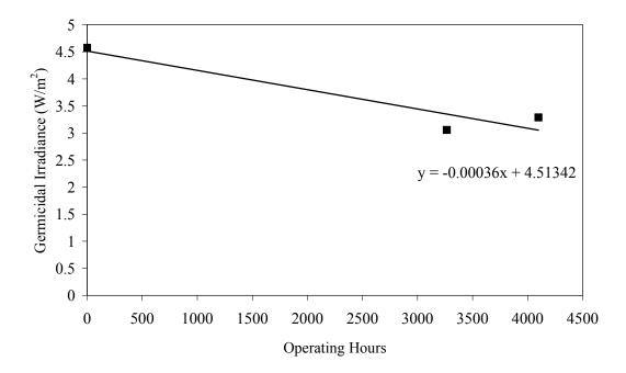
Figure 4.52 Germicidal irradiance as a function of operating hours with Type 1 MP lamps
