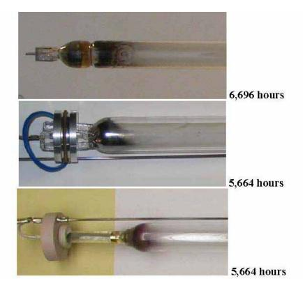
Figure 4.10 End darkening in LPHO lamps (top photo) and MP lamps (middle and bottom photos)
