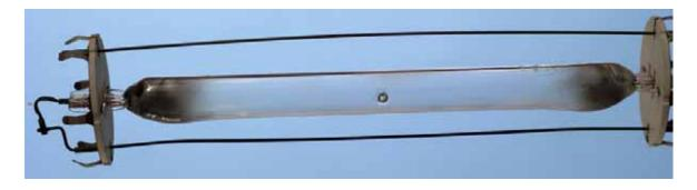
Figure 4.13 Lamp end distortion with a MP lamp with lamp end darkening
