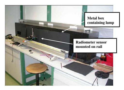
Figure 4.4 Apparatus used to measure spectral UV irradiance
