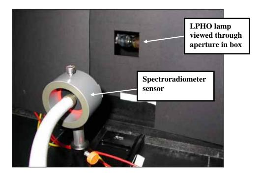
Figure 4.5 Mounting of the spectroradiometer sensor used to measure spectral irradiance with the LPHO lamp
