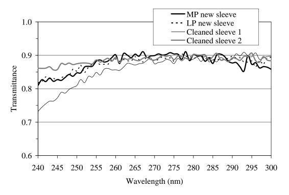
Figure 8.21 Transmittance of new quartz sleeve samples taken from replacement sleeves that were never used, and the transmittance of the two sleeve samples after cleaning with mild phosphoric acid bathroom cleaner
