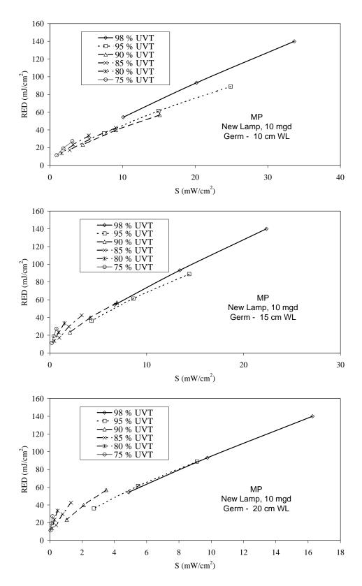
Figure 6.14 (Continued). MS2 RED (D10 =  $18 \text{ mJ/cm}^2$ ) as a function of DVGW UV sensor readings and UVT for water layers of 2, 5, 10, 15, and 20 cm
