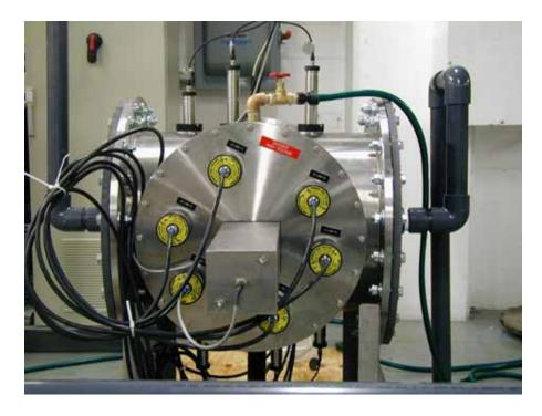
Figure 8.3 Photograph of the IDI reactor equipped with six 6 kW MP lamps
