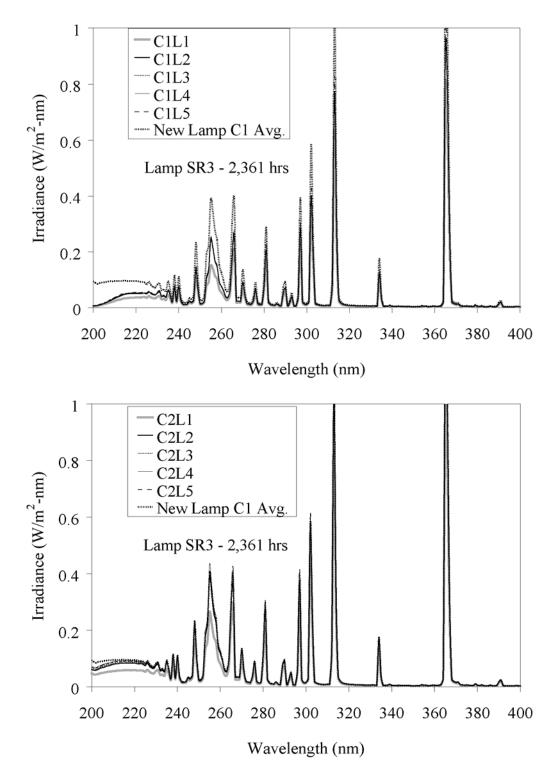
Figure 4.60 Spectral irradiance of Type 2 MP lamp SR3 aged 2,361 hours as a function of location along the lamp length and around the circumference (C1 - top, C2 - bottom)
