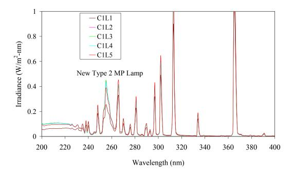
Figure 4.54 Spectral irradiance of the new Type 2 MP lamp as a function of location along the lamp length at location  ${\rm C1}$
