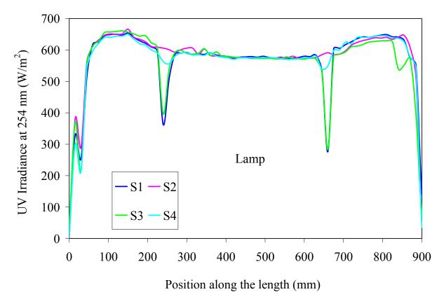
Figure 4.27 UV output at 254 nm of LPHO lamp #2 (432 hours) as a function of position along the length and around the circumference of the lamp
