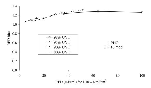
Figure 6.9 RED bias with the 6-row LPHO reactor as a function of RED based on  $D10 = 4 \text{ mJ/cm}^2$ . RED bias is calculated as the ratio of REDs for D10 = 18 and  $4 \text{ mJ/cm}^2$ .
