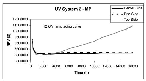
Figure 9.10 Impact of lamp replacement interval on life-cycle costs for the modeled UV systems, Analysis uses lamp-aging curves from data measured in this project, power costs of \$0.15/kW-hr, no dose pacing, and reactor capital costs varying with Lamp Aging Factor
