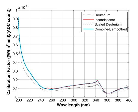
Figure 8.10 Spectrometer calibration curves
