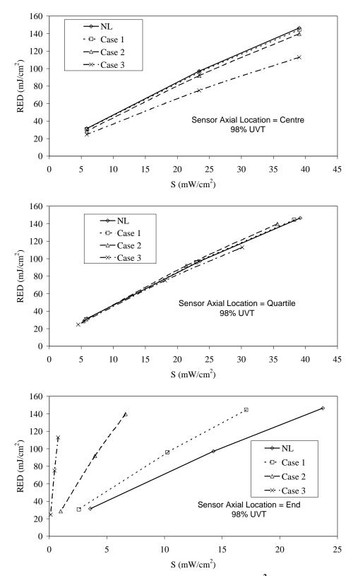
Figure 6.23 Relation between MS2 RED (D10 =  $18 \text{ mJ/cm}^2$ ) and DVGW UV sensor readings at 98% UVT for different cases of non-uniform MP lamp aging along the lamp length
