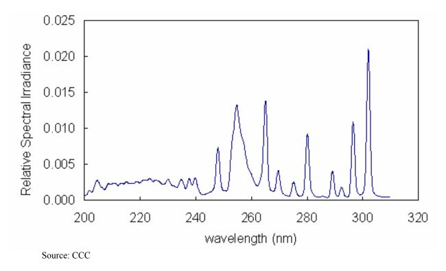
Figure 5.2 Spectral output of a new lamp for the Sentinel UV reactor
