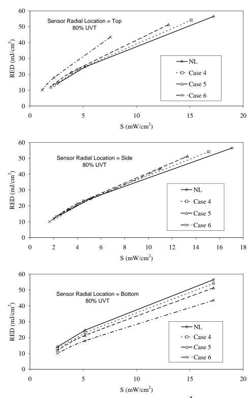
Figure 6.26 Relation between MS2 RED (D10 =  $18~mJ/cm^2$ ) and DVGW UV sensor readings at 80% UVT for different cases of non-uniform MP lamp aging about the lamp circumference
