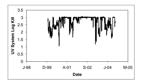
Figure 7.9 Pathogen log inactivation over time predicted by the Advanced LCA UVCAT tool
