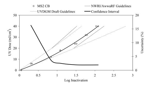
Figure 5.7 UV dose-response of MS2 phage measured during testing
