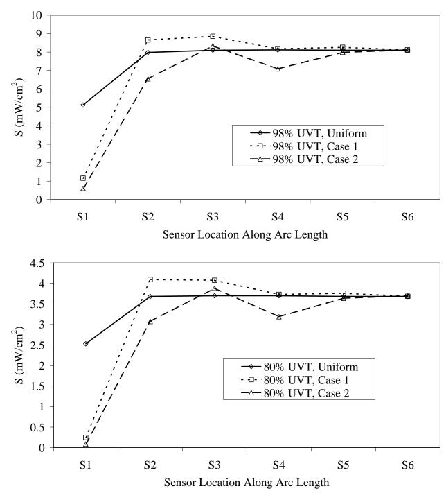
Figure 6.28 Impact of non-uniform LPHO lamp output along the lamp length on UV sensor readings (location S1 - lamp end, location S6 - center of the lamp, spacing between UV sensors - 15~cm)
