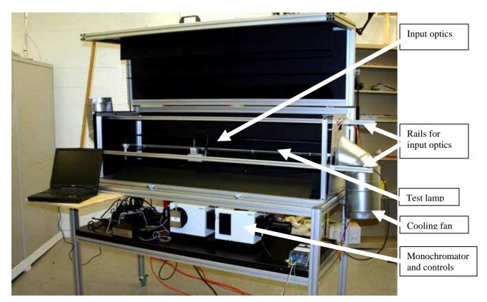
Figure 8.7 Photograph of the measurement chamber
