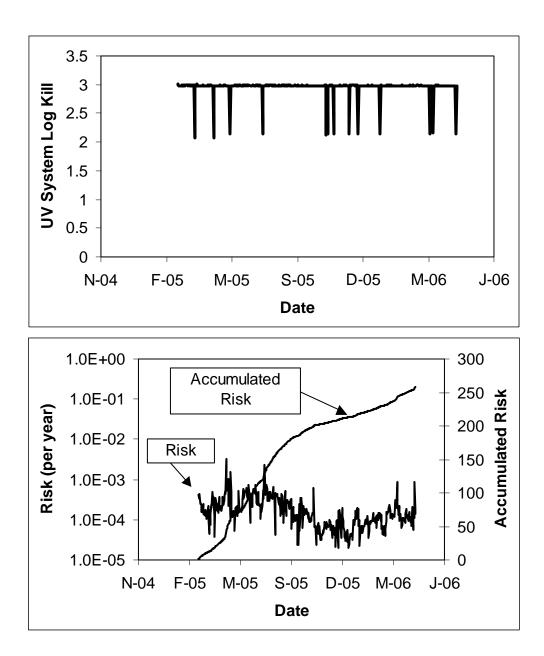
Figure 12.13 UV system log inactivation (top), and annual infection risk and accumulated infection (bottom) for the Case 4 LPHO system
