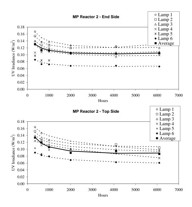
Figure 8.14 (Continued) Lamp aging data for the UV reactor equipped with six 6.0-kW MP lamps - Lamps 1, 2, 3, 4, 5 and 6 were operated at 6.0, 6.0, 5.5, 5.0, 4.0, and 3.5 kW, respectively; Average excludes lamp 5
