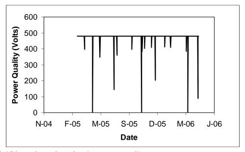
Figure 12.6 Line voltage data showing power quality events
