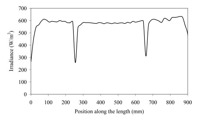
Figure 4.25 UV output at 254 nm of a new amalgam LPHO lamp as a function of position along the length of the lamp
