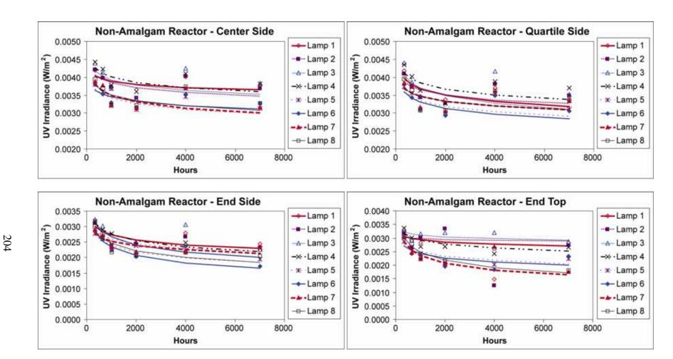
Figure 8.19 Lamp aging data for the UV reactor equipped with eight 130-W non-amalgam LPHO amps. Lamps 1 through 4 operated at 100% power; Lamps 5 through 8 operated at 80% power
