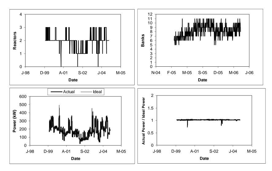
Figure 10.8 Case 1: UV system consisting of three 2-bank reactors: reactors on (top left), banks on (top right), power consumption (bottom left), and ratio of ideal-to-actual power (bottom right)
