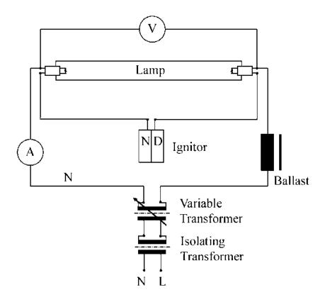
Figure 4.2 Schematic of the LPHO lamp power supply and ballast
