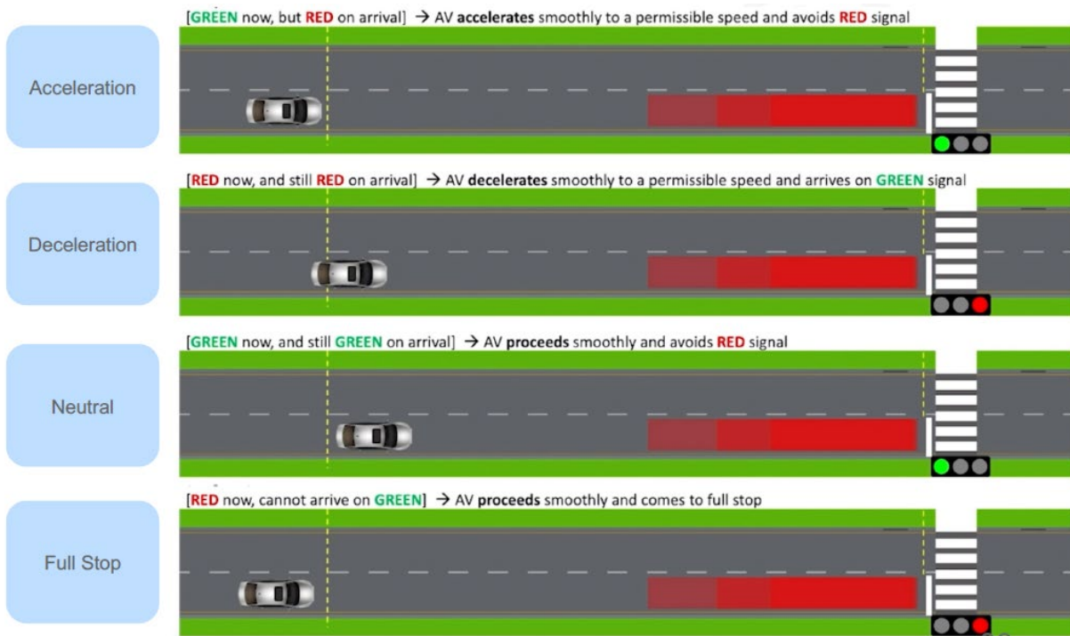
Figure 10. The Four Scenarios of a CAV Approaching a Signalized Intersection
