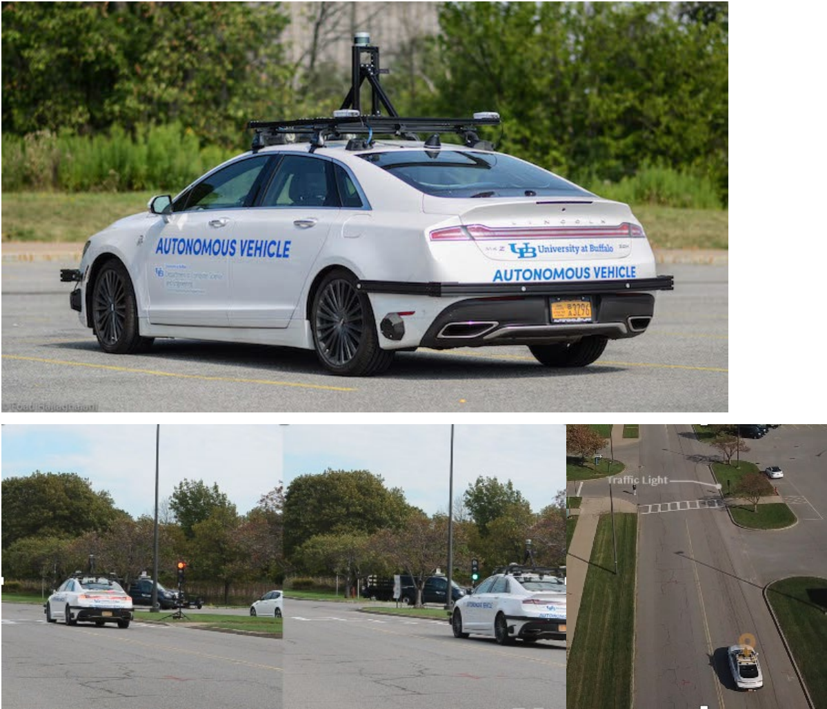
Figure 13. The Test Scenarios Using a CAV Platform (Lincoln MKZ) and Portable Traffic Light System
