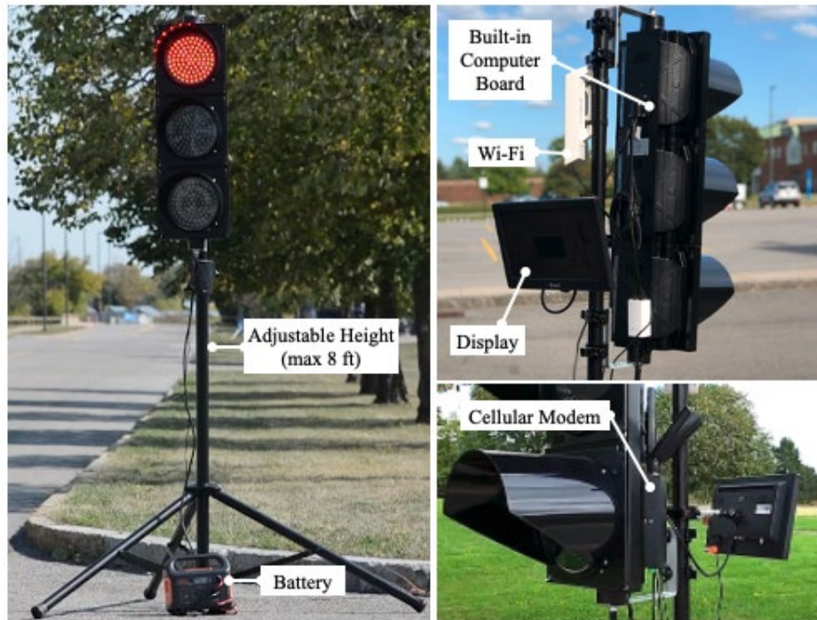
Figure 4. The Structure of a Portable Traffic Signal
