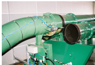
Figure 1-4. Two-Way Diverter Valve (Source: Kogler, 2007)
