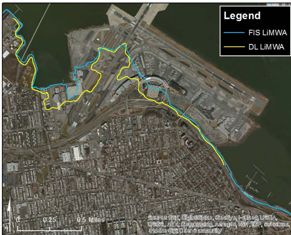
Figure 8. Comparison of FIS LiMWA and DL-derived LiMWA at Test Location
