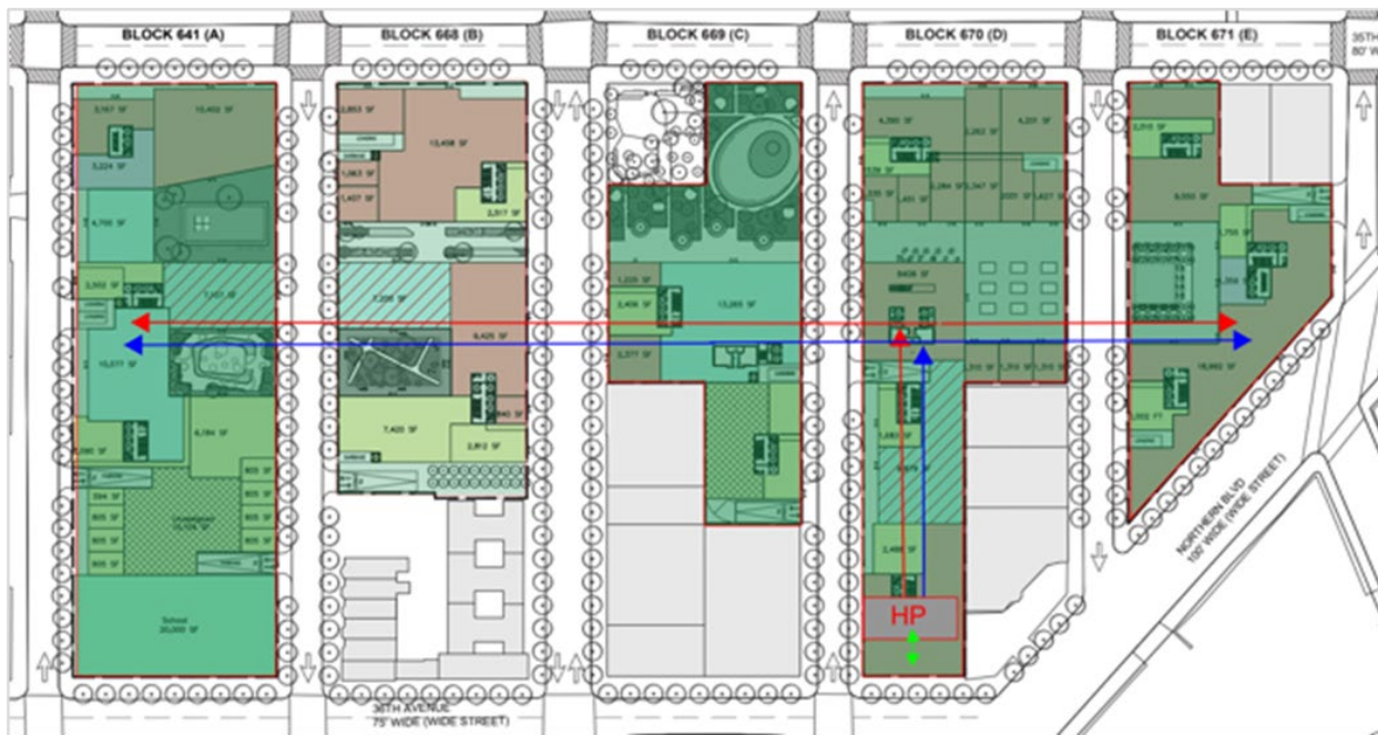
Figure 10. Single Central Plant Serving Two Districts
