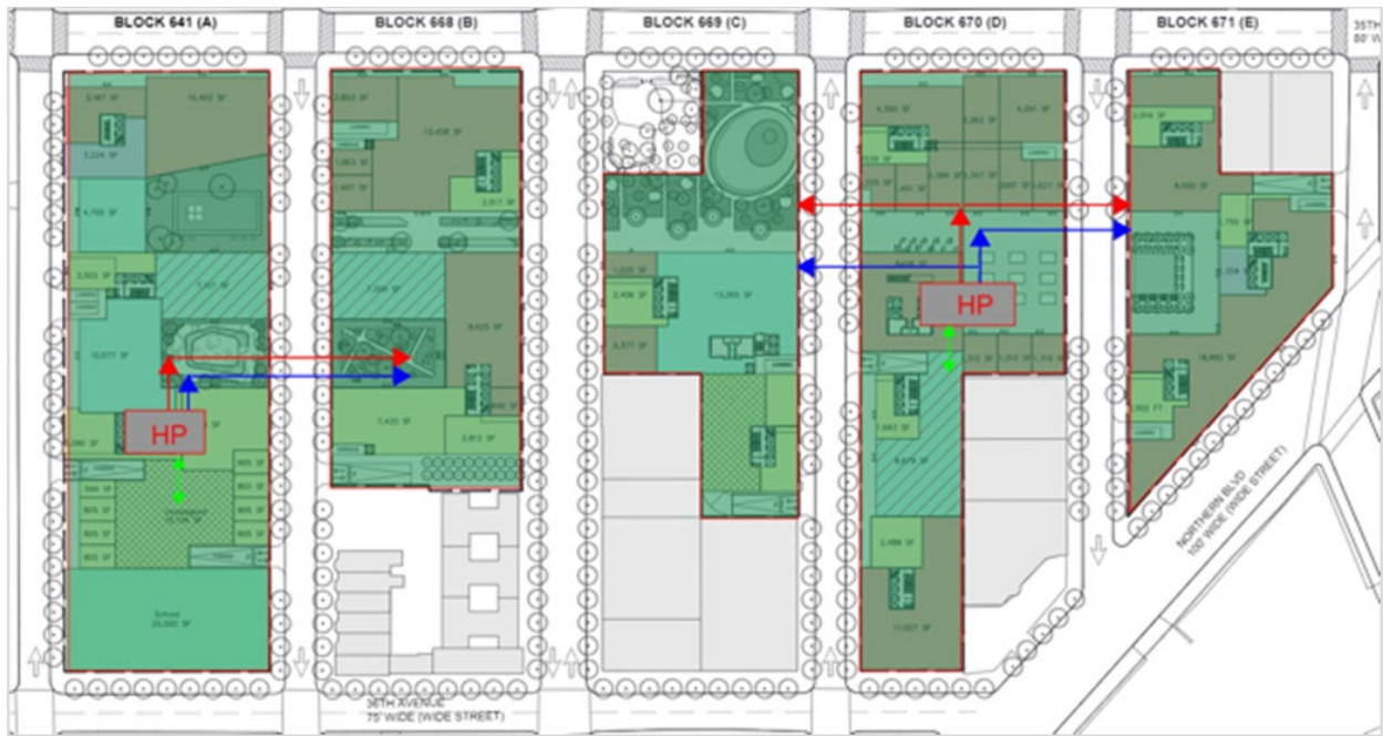
Figure 11. Two Central Plants Serving Two Independent Districts
