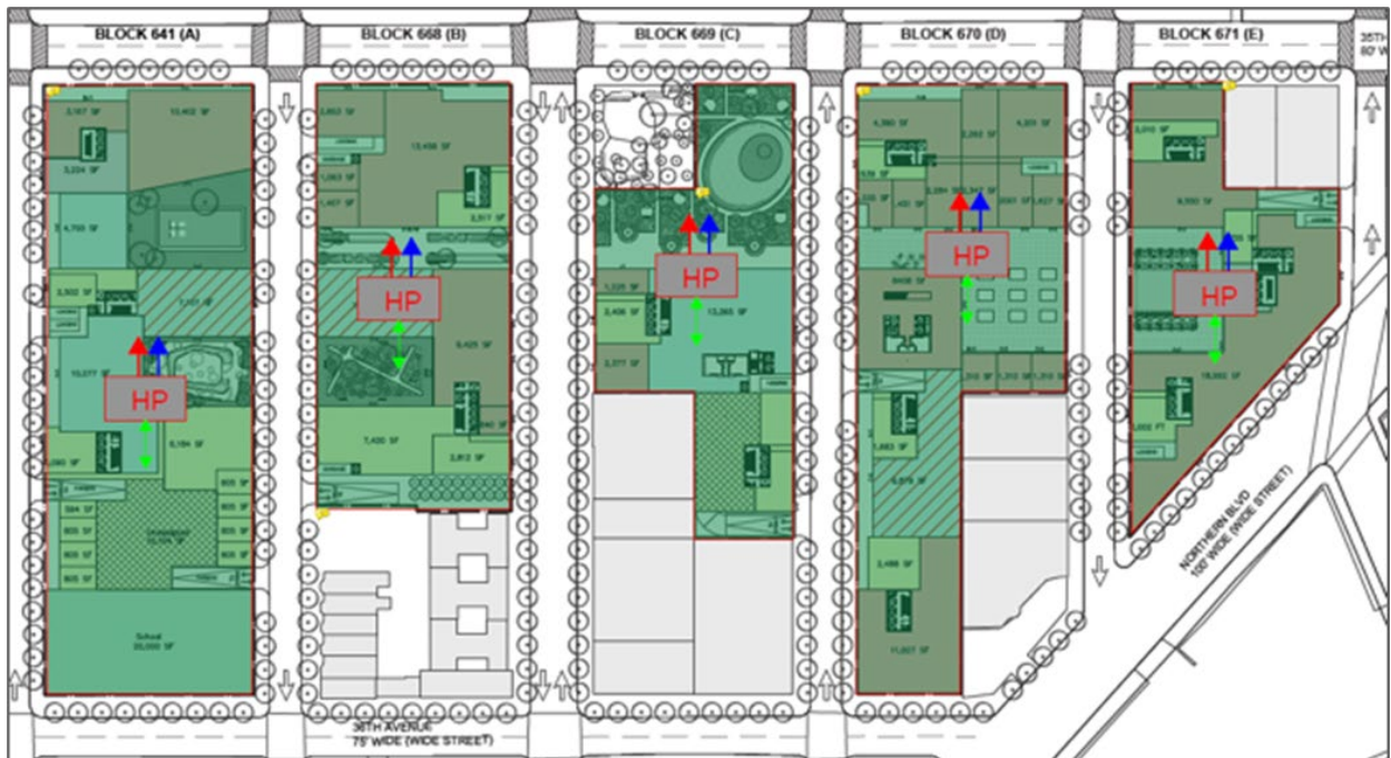
Figure 12. Decentralized Heat Pump Configuration
