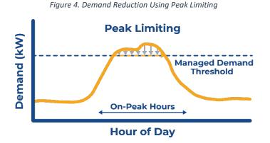
Load shedding entails reducing or turning off loadsduring the on-peak hours to keep the aggregated demand below the preset level. The candidates for shedding should only be loads that can be reduced or turned off without affecting occupant safety, loads that will not lead to an unrecoverable impact on
