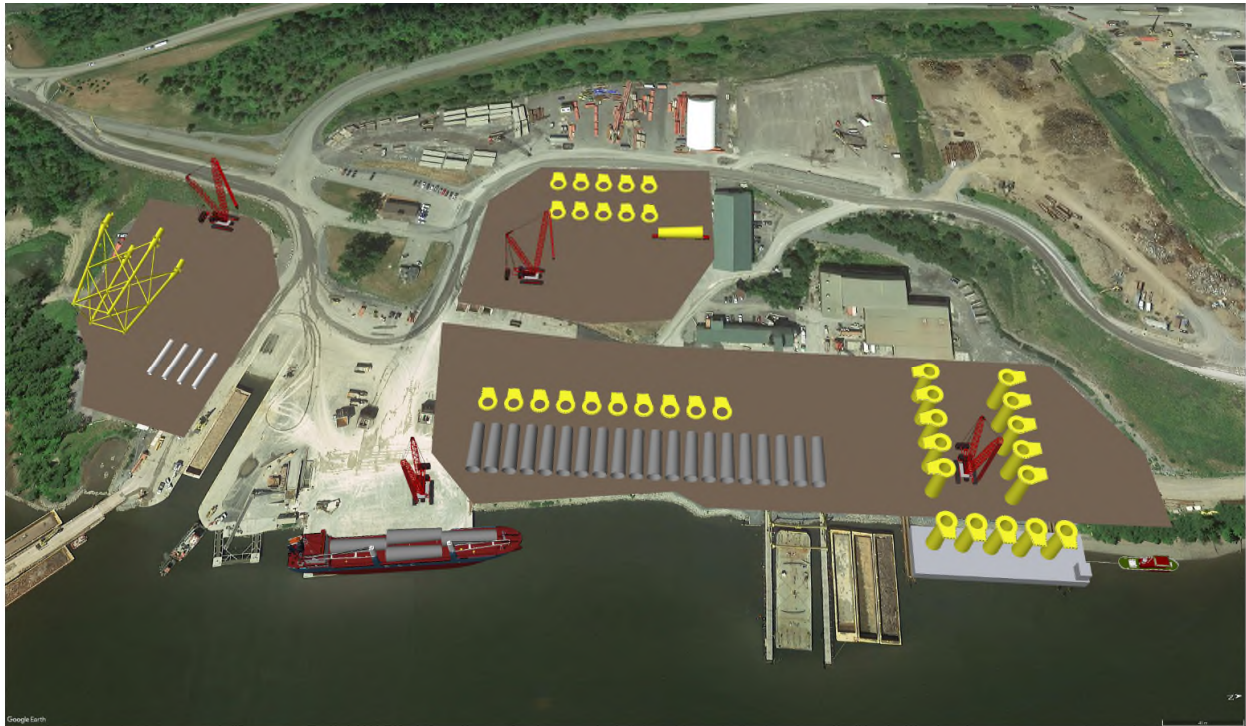
Figure 1.1-4 Steel Work for Foundation Components at Port of Coeymans
