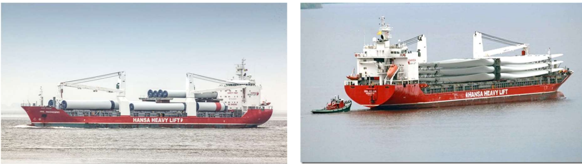
Figure 11.3-14 Heavy Transport Vessels carrying WTG components
