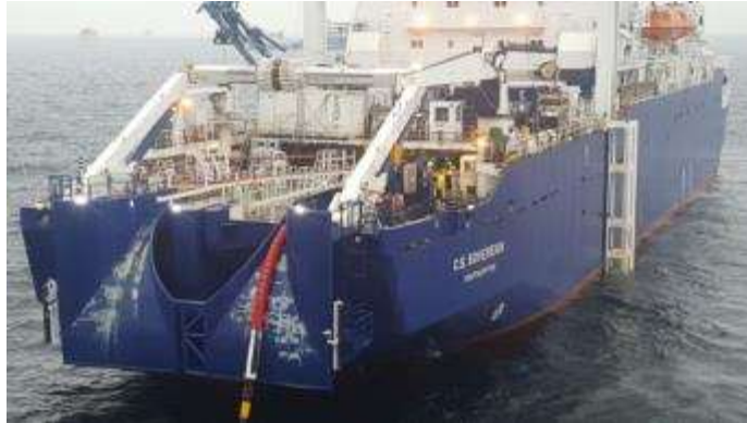
Figure 11.3-12 Inter-array Cable Installation Vessel
