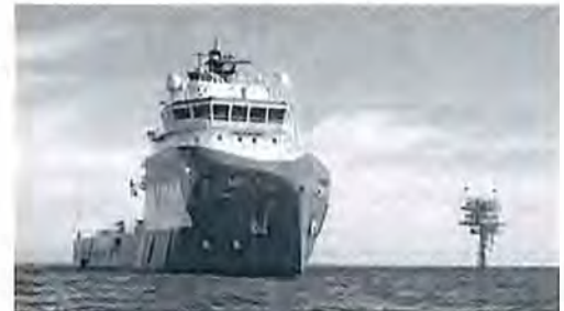
Kroonborg is the first offshore vessel in the world to sail on GTL fuel, a liquid fuel made of natural gas with less emissions than conventional fuels for vessels.
